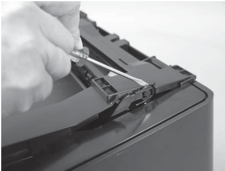
Figure 1-23 Remove the cartridge door (1 of 3)
