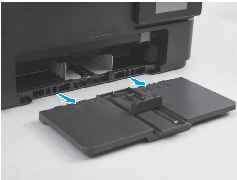
Figure 1-5 Remove the input tray
