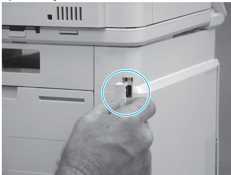
Figure 1-62 Align the tabs on the cover
