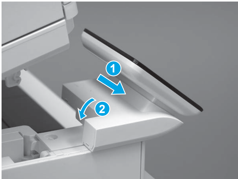
Figure 1-2210 Install the control-panel cable cover
