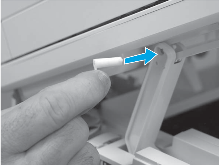
Figure 1-1010 Install the slider pin
