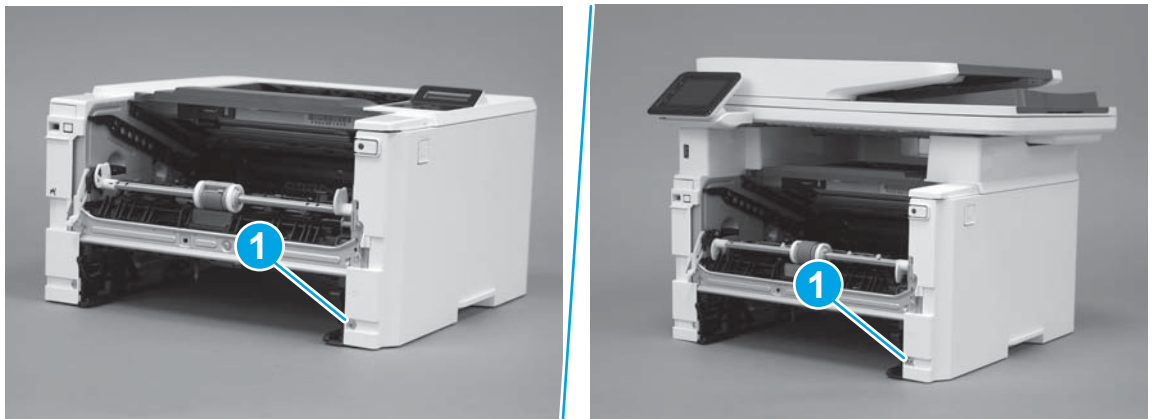
Figure 1-1018 Install one screw
