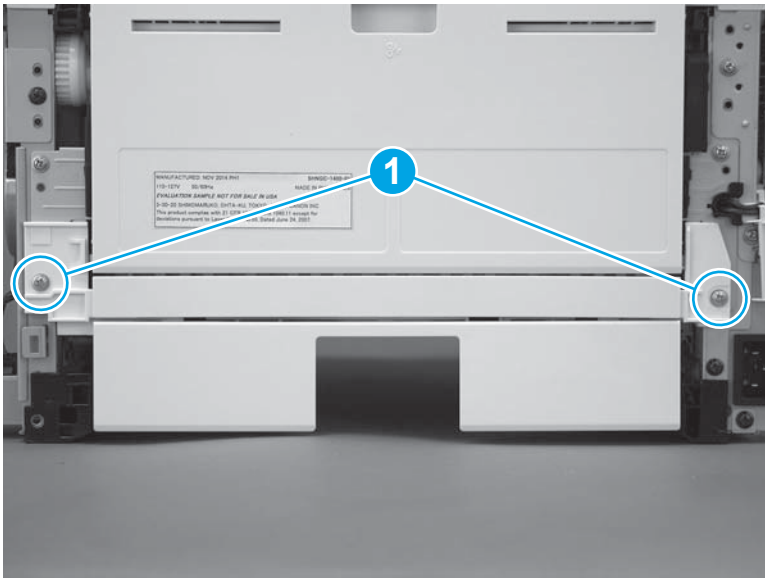
Figure 1-710 Install two screws
