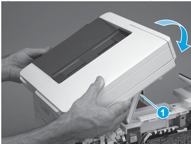
Figure 1-1187 Rotate the ISA towards the front of the printer
