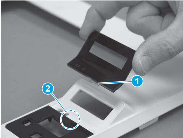
Figure 1-423 Position the operator cover on the printer
