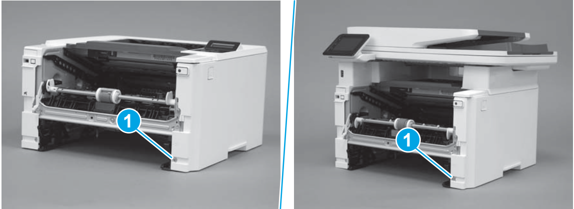
Figure 1-392 Install one screw
