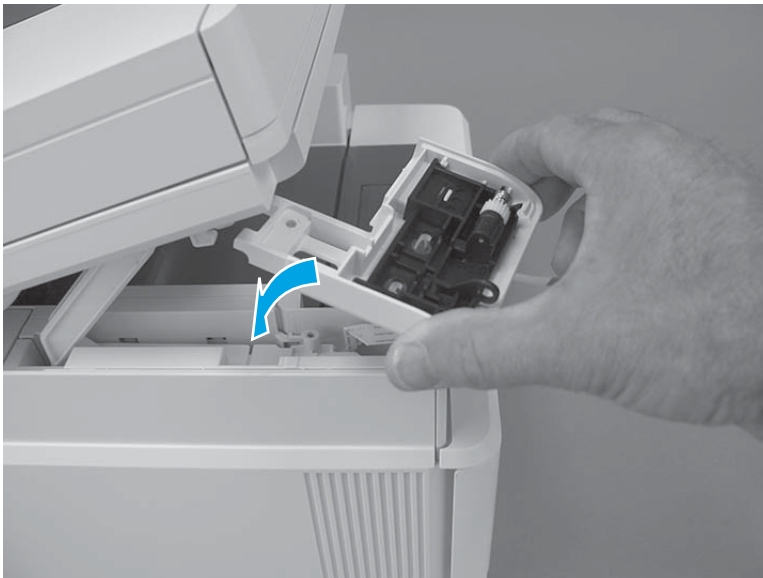
Figure 1-2202 Install the control panel mount base
