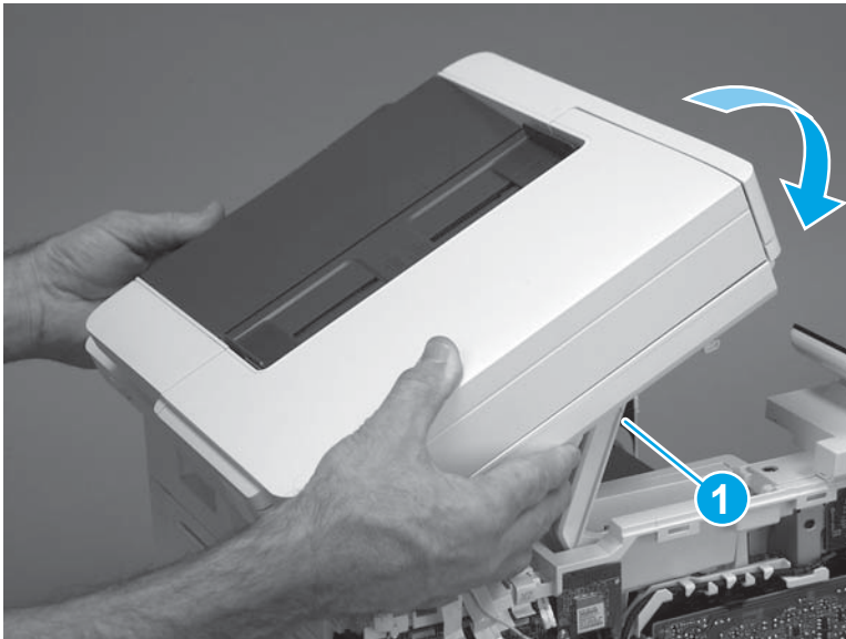
Figure 1-1095 Rotate the ISA towards the front of the printer
