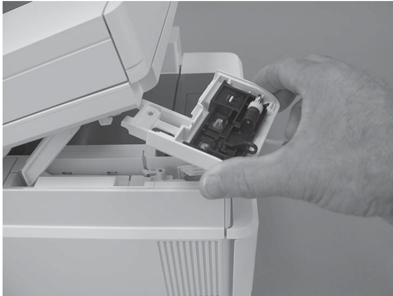
Figure 1-2168 Release the control panel mount base
