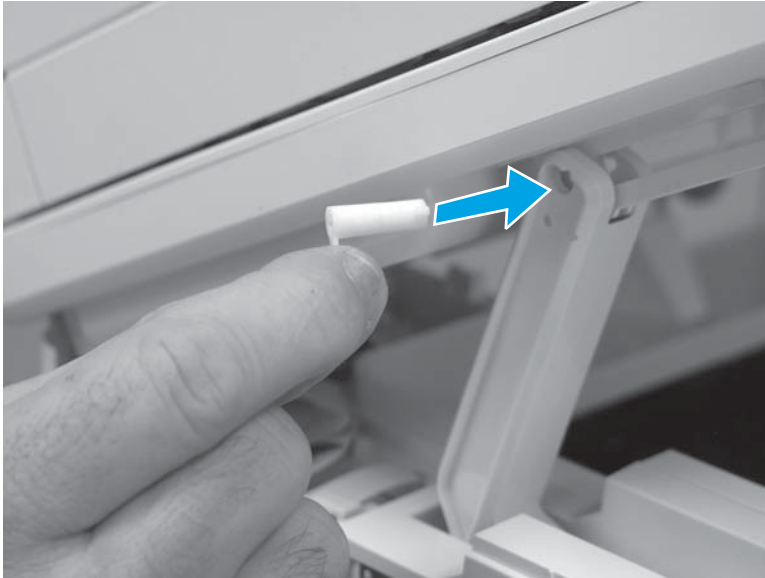
Figure 1-1098 Install the slider pin
