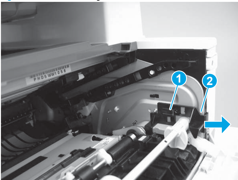
Figure 1-1449 Remove the guide
