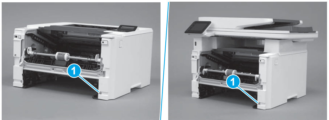
Figure 1-607 Install one screw
