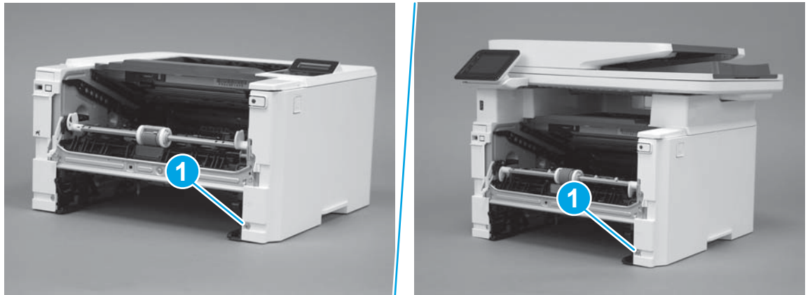
Figure 1-1950 Install one screw
