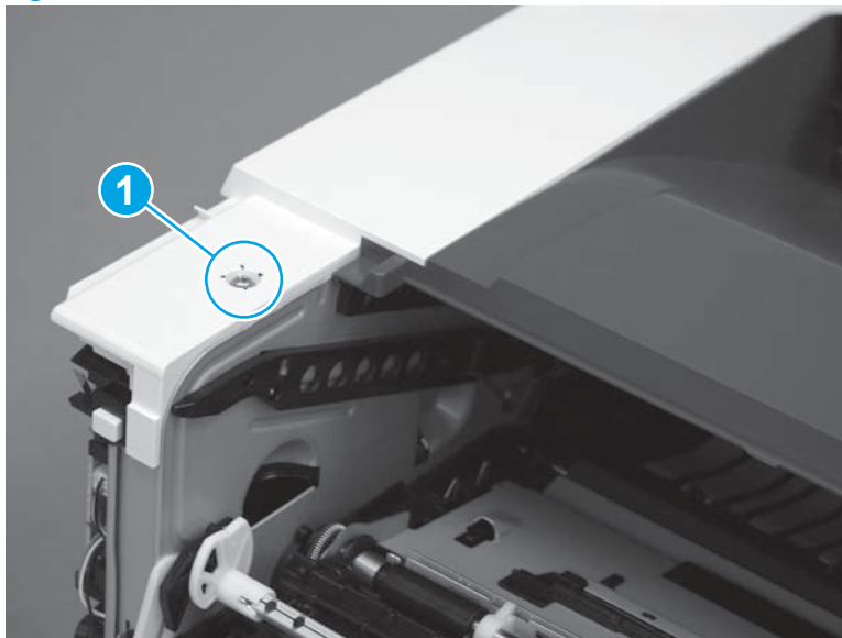
Figure 1-2078 Install one screw
