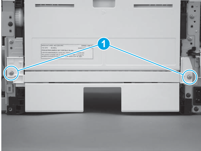
Figure 1-160 Install two screws
