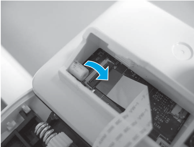
Figure 1-2205 Connect the FFC
