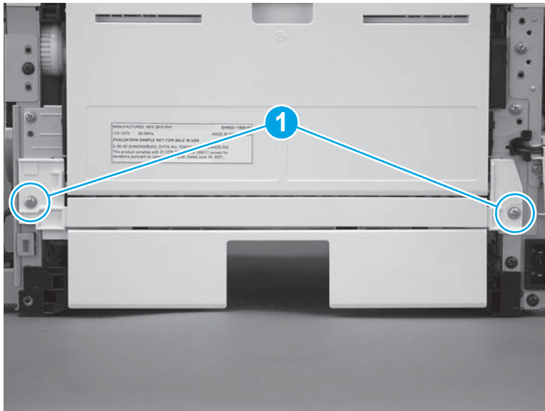
Figure 1-196 Install two screws
