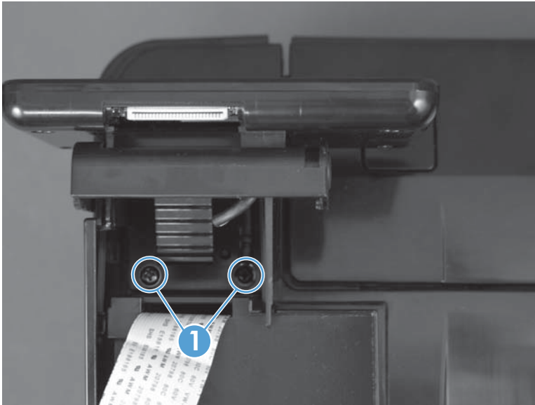
Figure 1-20 Remove the control panel (2 of 3)
