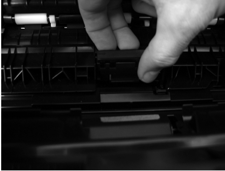
Figure 1-8 Remove the MP tray separation pad (5 of 5)
