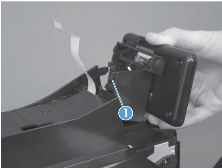
Figure 1-21 Remove the control panel (3 of 3)
