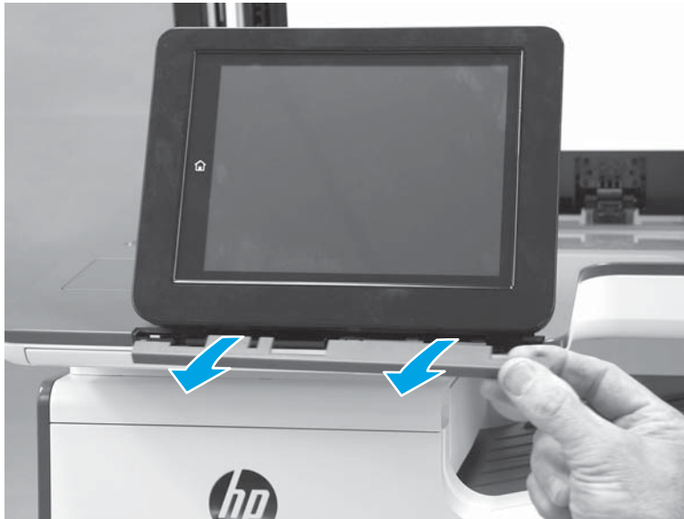
Figure 1-197 Remove the cover
