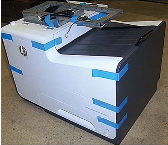
Figure 1-784 Remove the shipping tape
