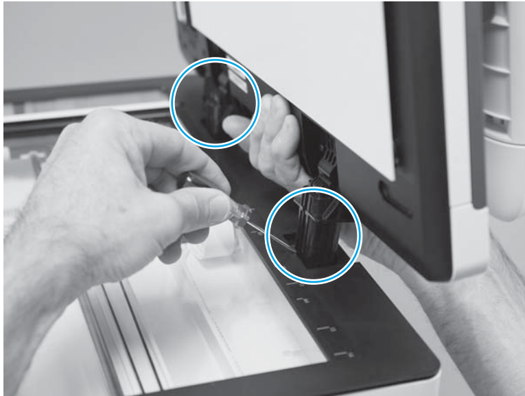
Figure 1-685 Release two tabs on the hinges
