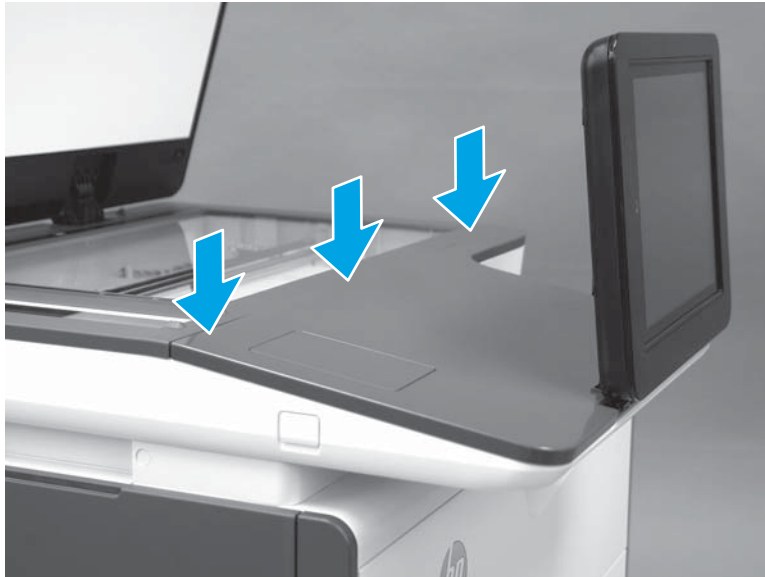
Figure 1-46 Engage three bosses
