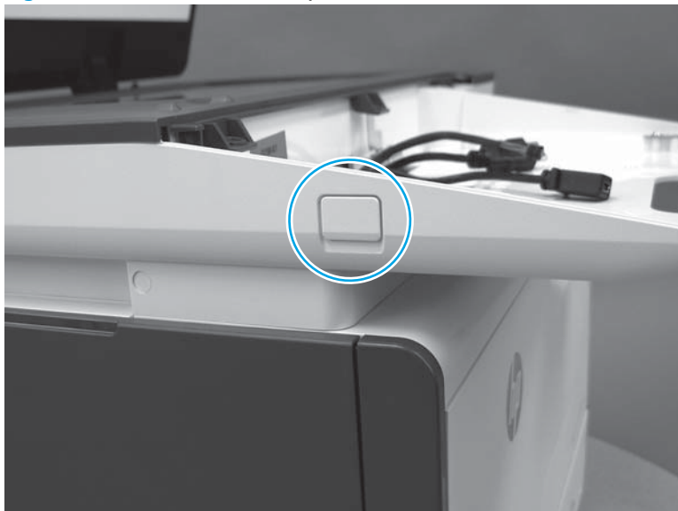
Figure 1-205 Remove the USB port cover
