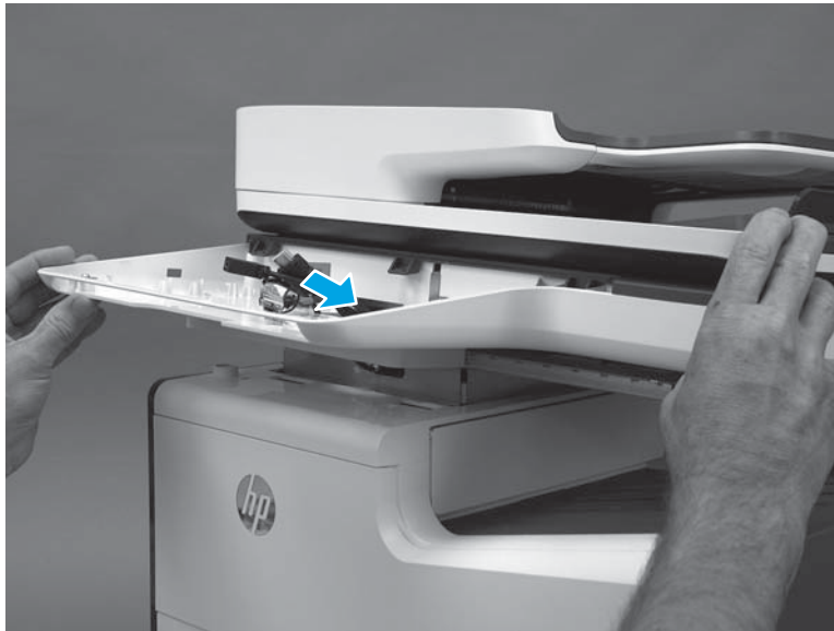
Figure 1-318 Pass the wire harnesses and cables through the opening
