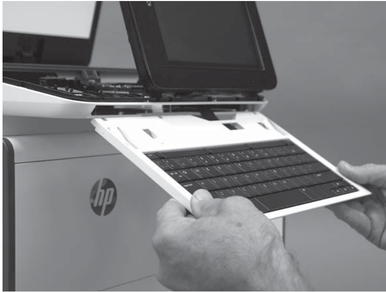
Figure 1-664 Remove the keyboard (586z)
