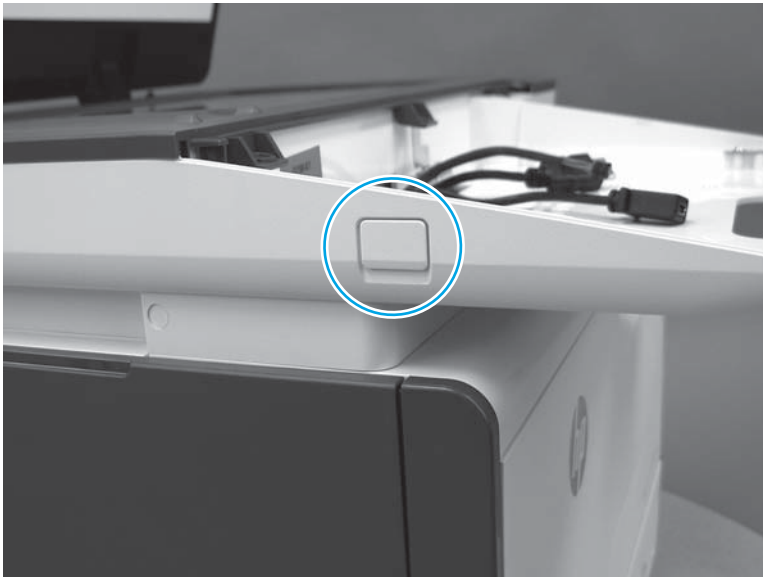
Figure 1-406 Install the USB port cover
