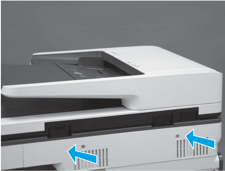
Figure 1-728 Install the SCB cover
