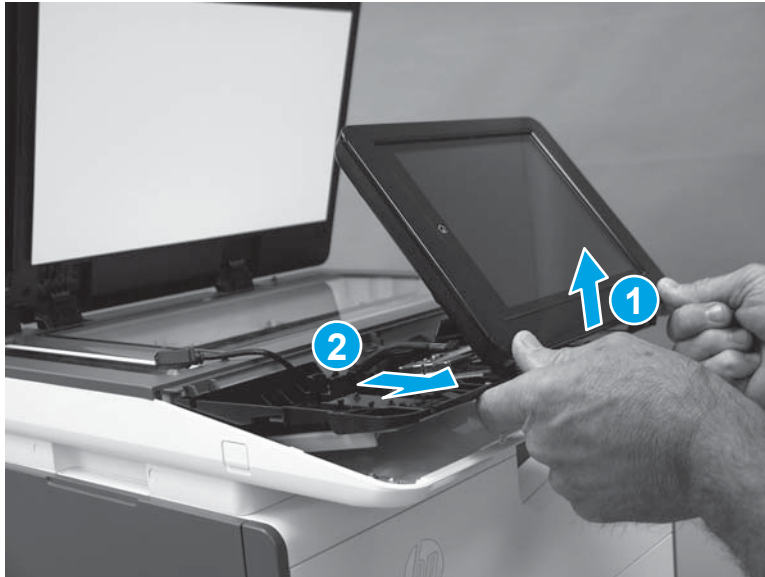
Figure 1-204 Remove the control panel
