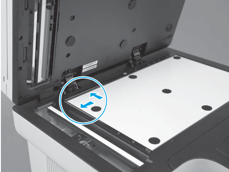
Figure 1-27 Place the white backing on the glass
