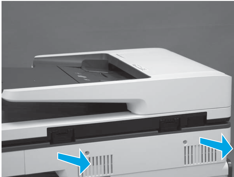
Figure 1-605 Remove the SCB cover
