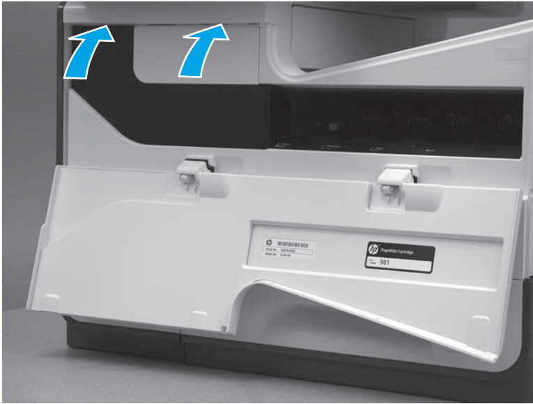
Figure 1-831 Close the blank cover
