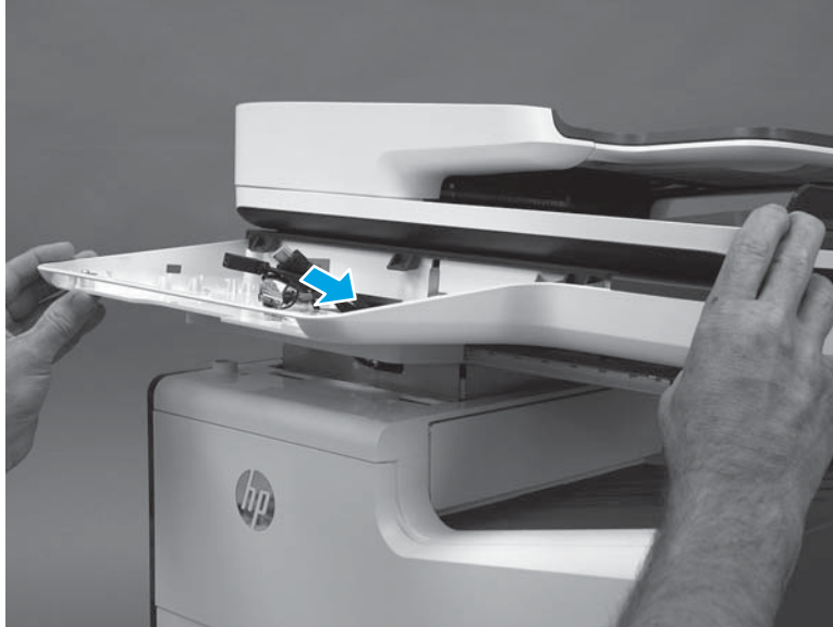
Figure 1-216 Pass the wire harnesses and cables through the opening
