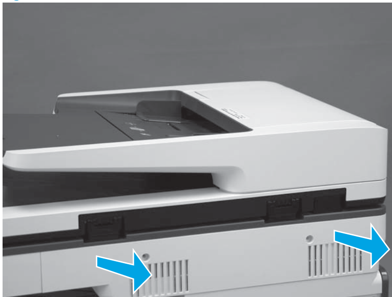
Figure 1-209 Remove the SCB cover
