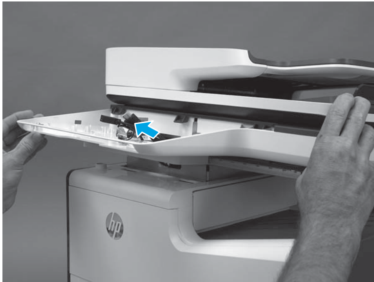
Figure 1-914 Pass the wire harnesses and cables through the opening
