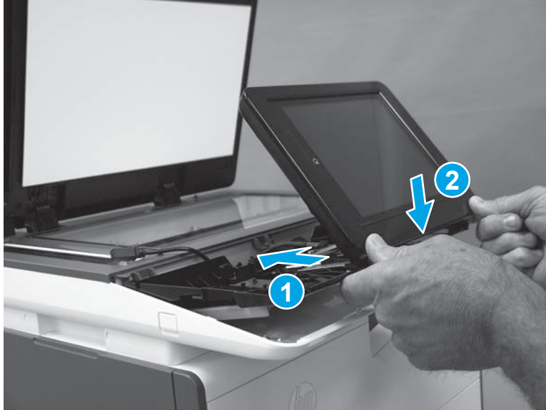
Figure 1-929 Install the control panel
