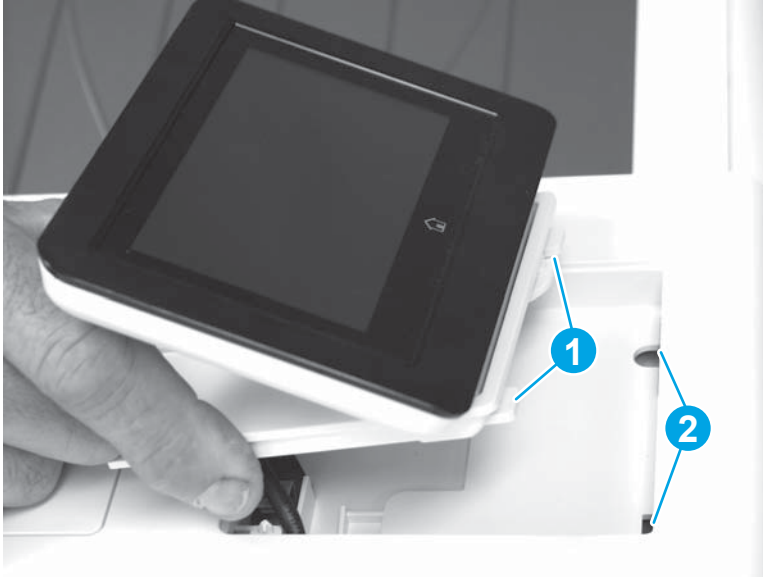
Figure 1-417 Install the control panel
