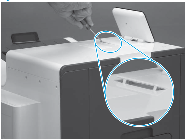
Figure 1-75 Release two tabs
