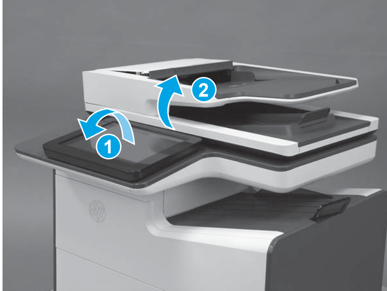
Figure 1-889 Tilt the control panel up
