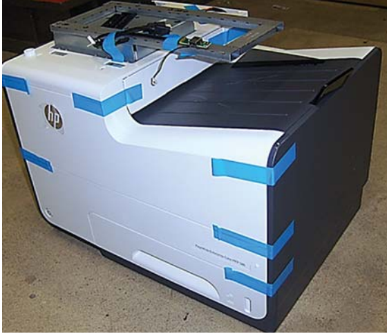
Figure 1-856 Remove the shipping tape
