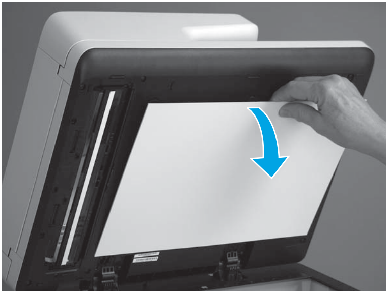
Figure 1-10 Remove the white backing
