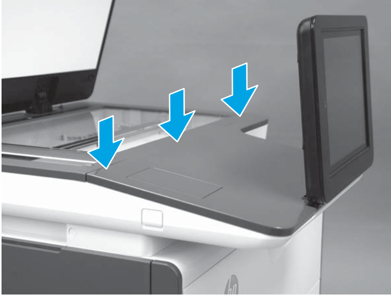
Figure 1-935 Install the control-panel cover
