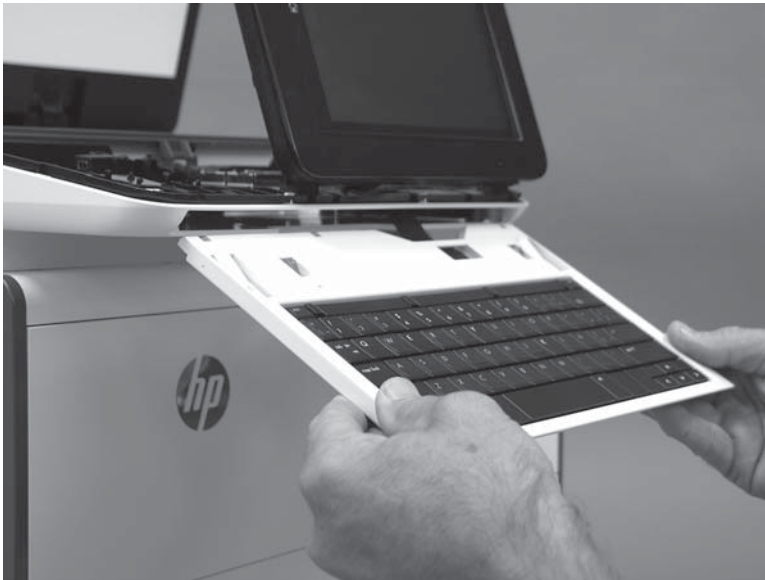
Figure 1-304 Remove the keyboard (586z)
