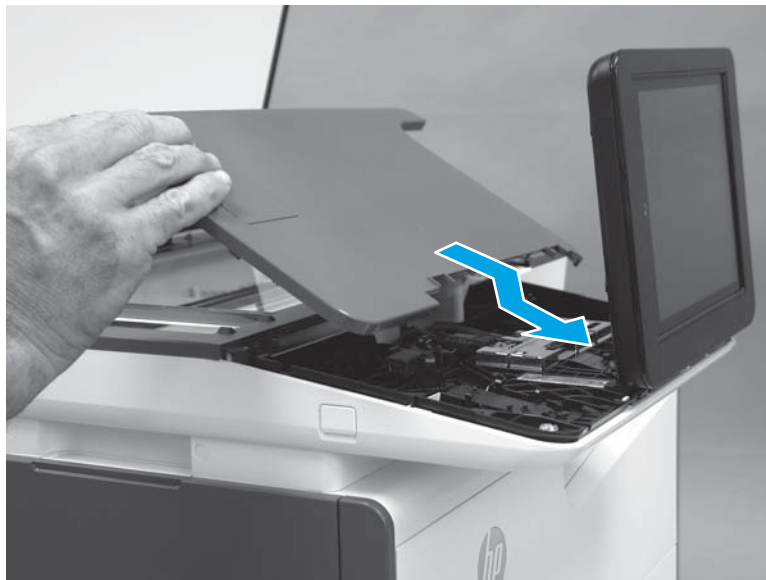
Figure 1-934 Install the cover
