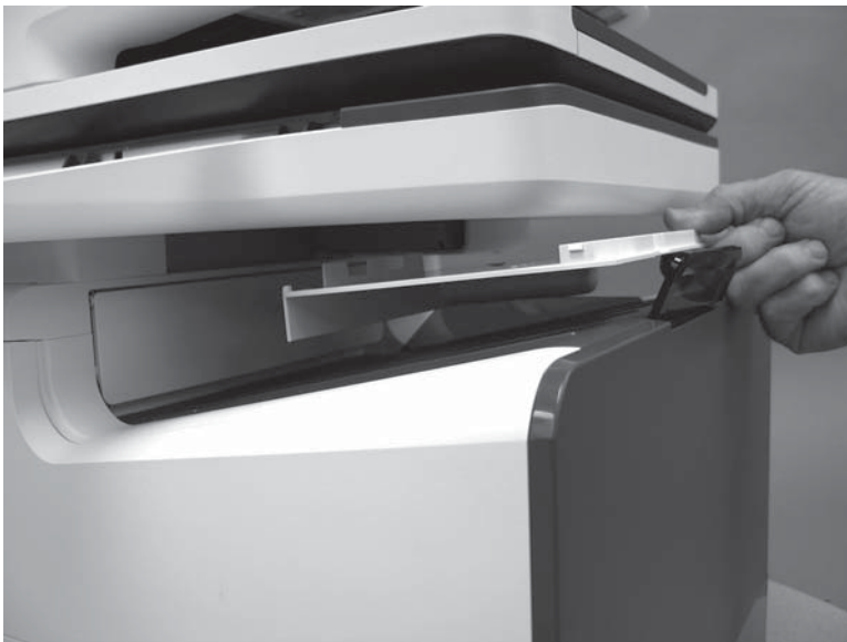
Figure 1-446 Remove the scanner base cover
