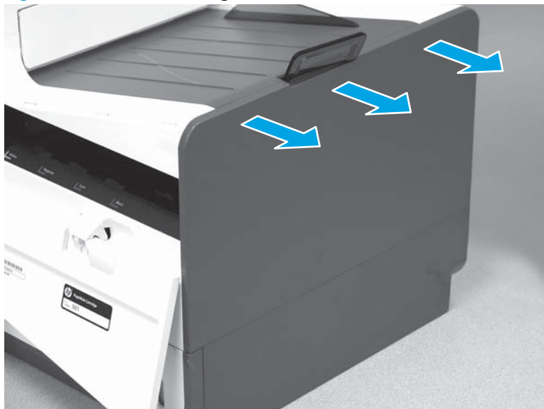
Figure 1-740 Release the right cover (outer)
