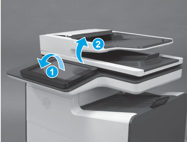
Figure 1-48 Tilt the control panel up
