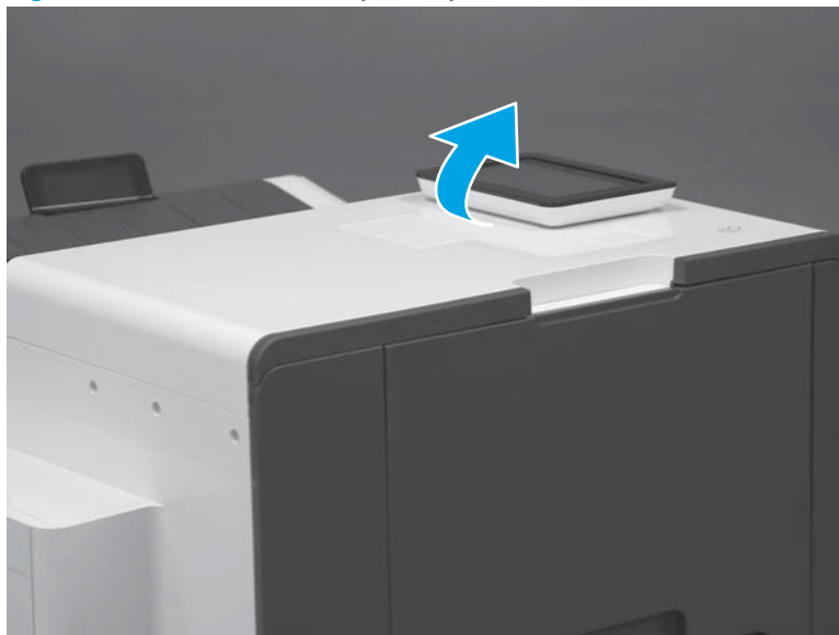
Figure 1-141 Tilt the control panel up
