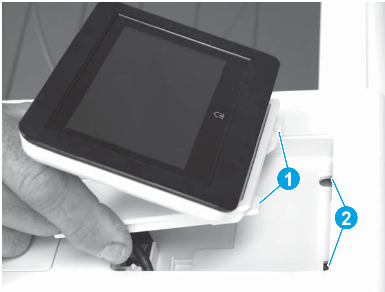
Figure 1-191 Install the control panel
