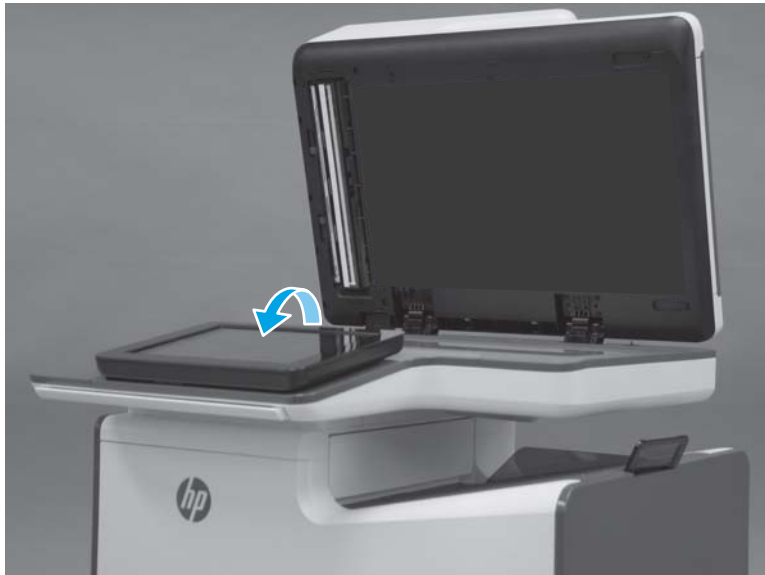
Figure 1-657 Tilt the control panel up
