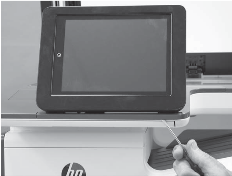
Figure 1-658 Release the small gray plastic cover
