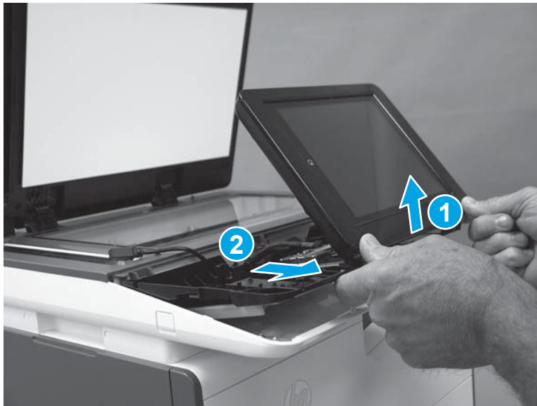
Figure 1-306 Remove the control panel
