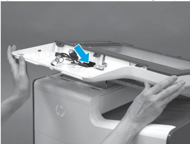
Figure 1-695 Pass the wire harnesses and cables through the opening
