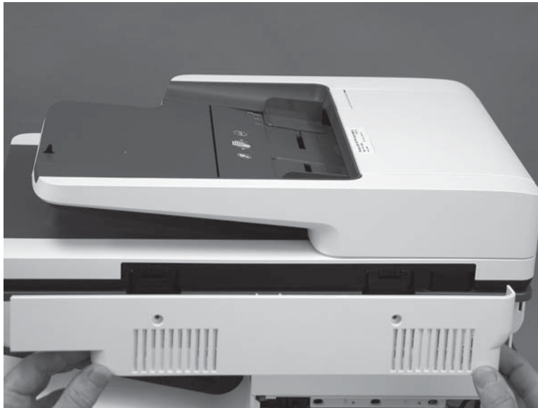
Figure 1-922 Align the tabs on the SCB cover
