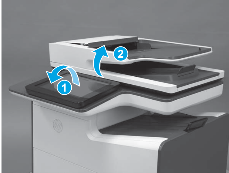
Figure 1-297 Tilt the control panel up
