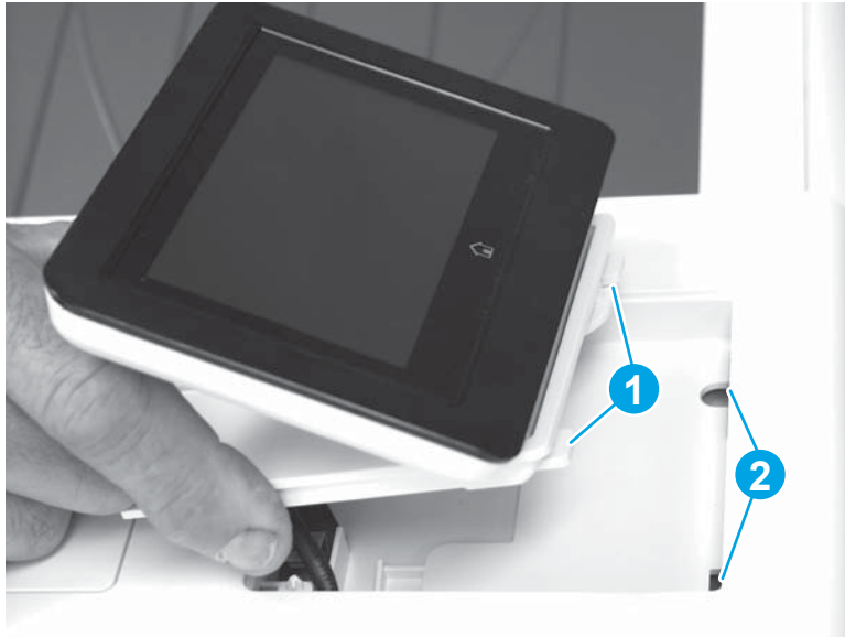
Figure 1-81 Install the control panel
