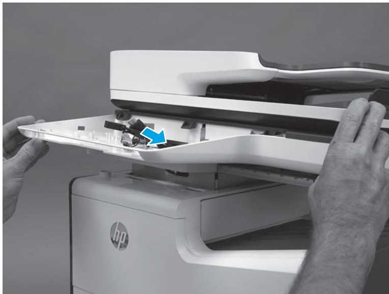
Figure 1-448 Pass the wire harnesses and cables through the opening
