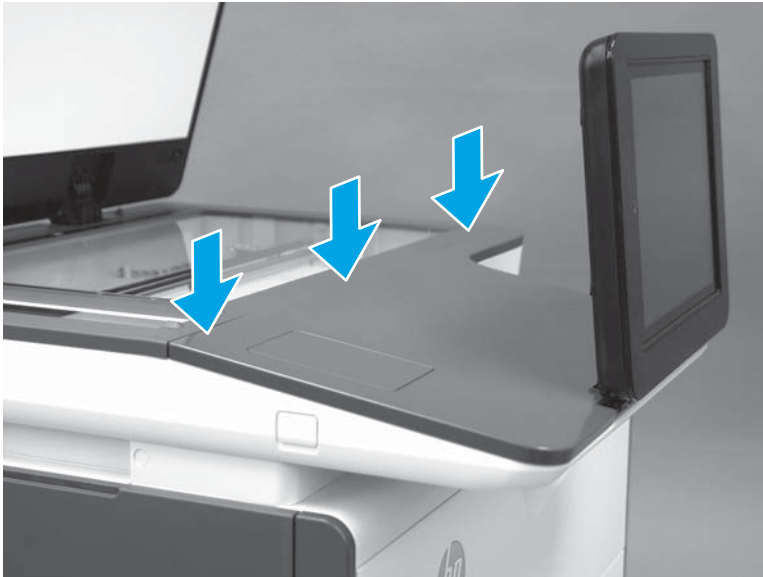
Figure 1-550 Install the control-panel cover
