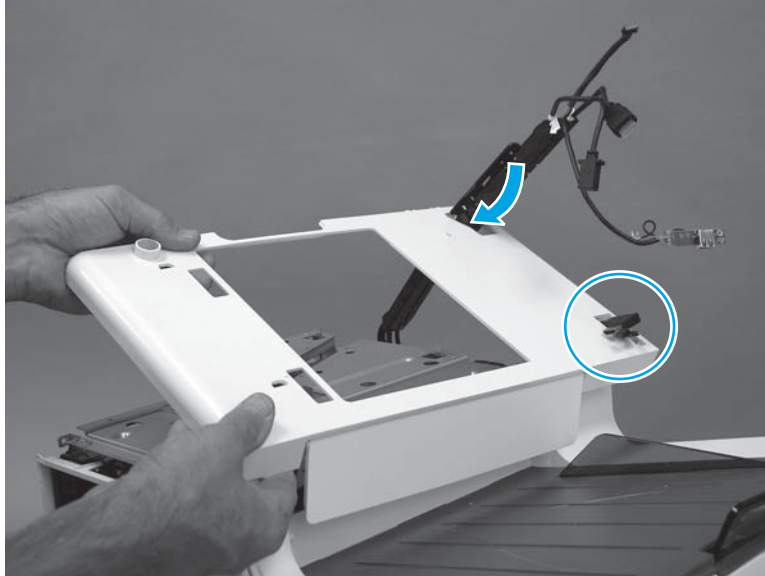
Figure 1-242 Install the top cover (586)
