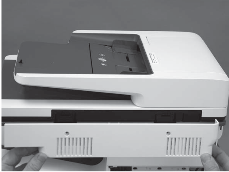
Figure 1-652 Align the SCB cover tabs and printer slots
