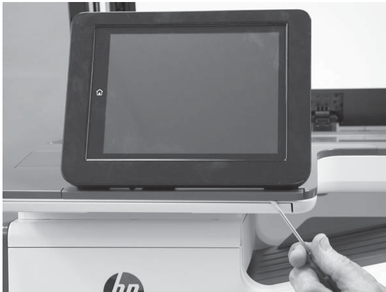
Figure 1-298 Release the small gray plastic cover
