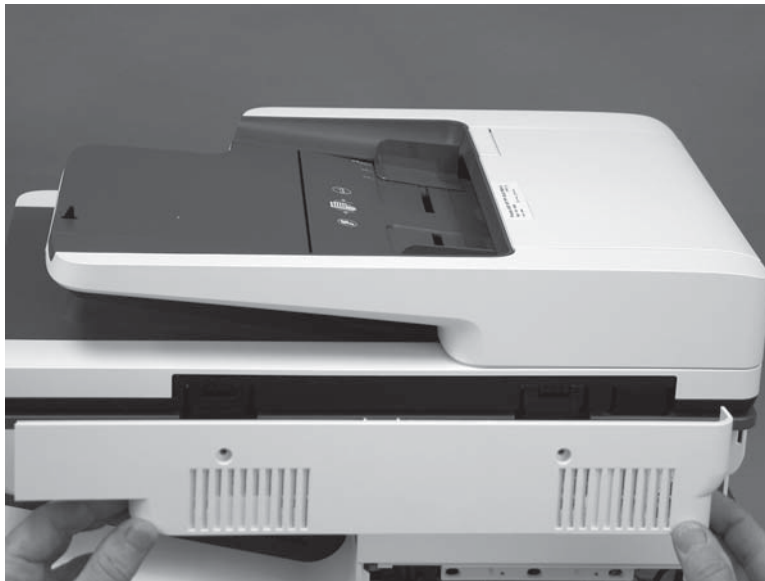
Figure 1-727 Align the SCB cover tabs and printer slots
