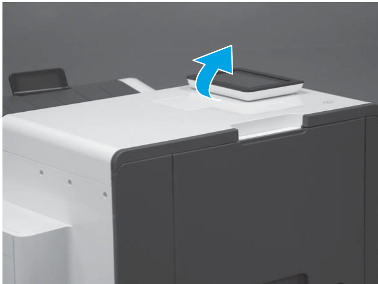
Figure 1-74 Tilt the control panel up
