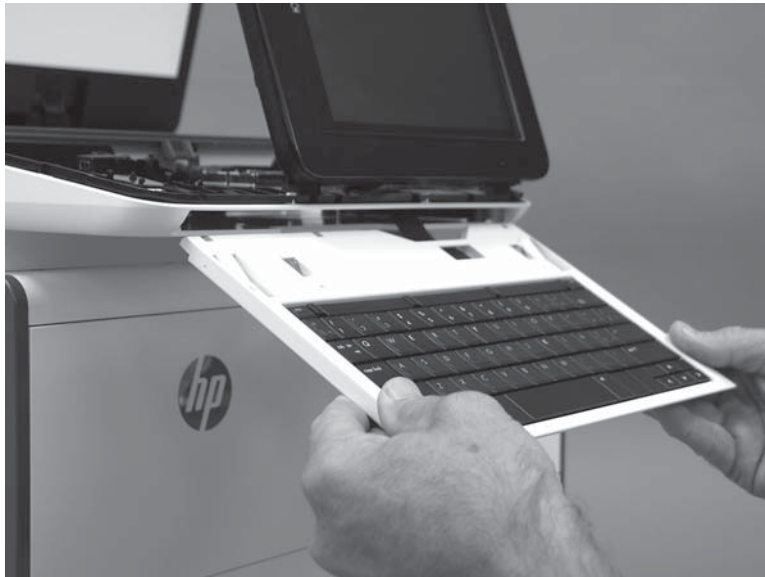
Figure 1-57 Install the keyboard
