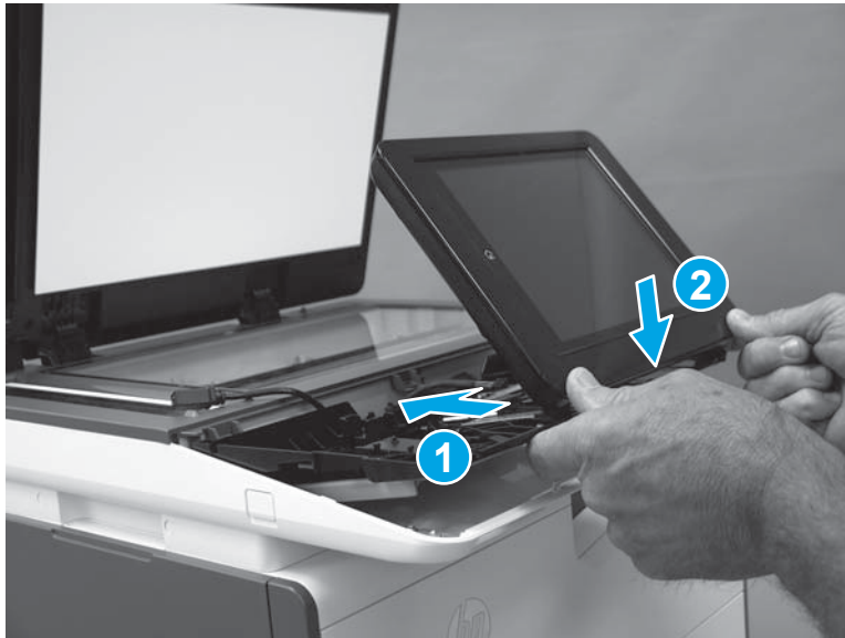
Figure 1-731 Install the control panel
