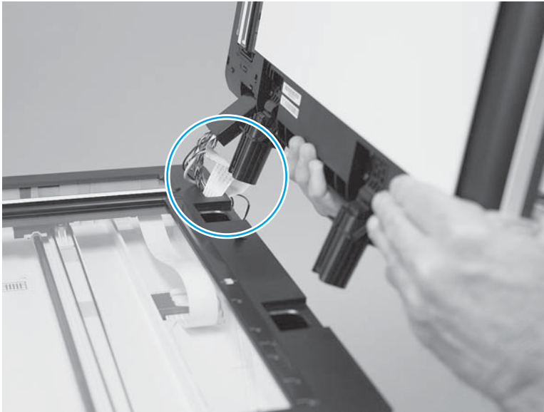
Figure 1-610 Remove the document feeder
