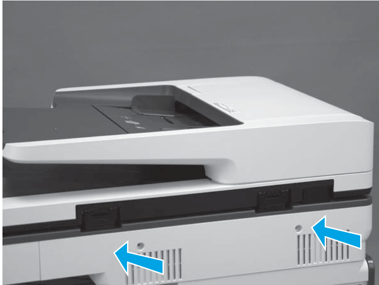
Figure 1-653 Install the SCB cover
