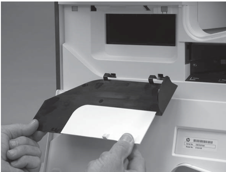
Figure 1-828 Install the blank cover
