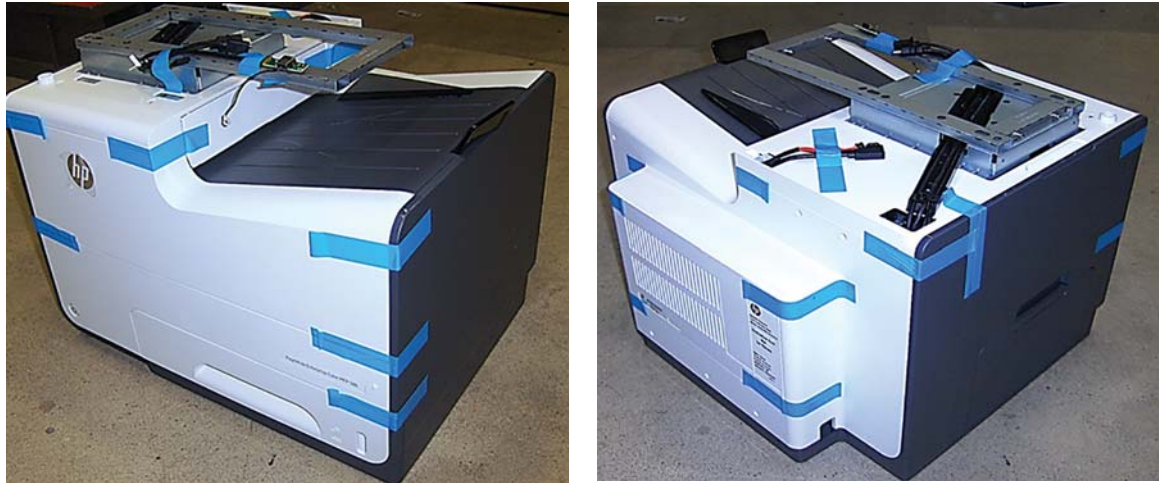
Figure 1-853 Box the DU for shipping
