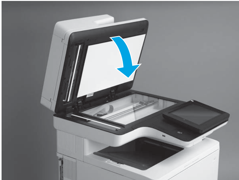
Figure 1-18 Close the document feeder
