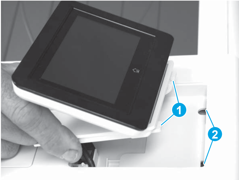
Figure 1-824 Install the control panel
