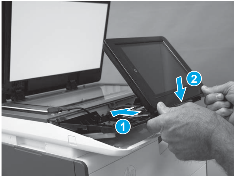
Figure 1-408 Install the control panel
