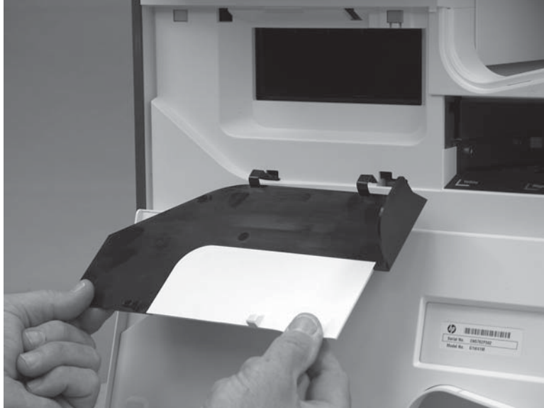
Figure 1-937 Install the blank cover
