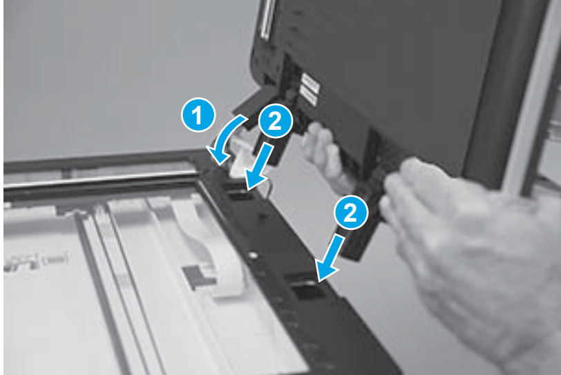
Figure 1-710 Install the document feeder
