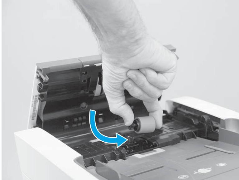
Figure 1-973 Install the roller assembly
