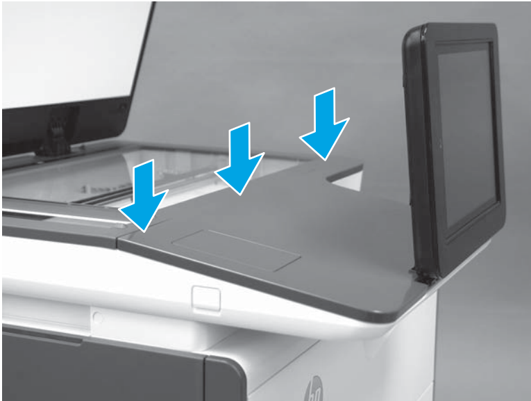
Figure 1-414 Install the control-panel cover
