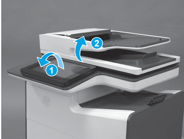
Figure 1-31 Tilt the control panel up
