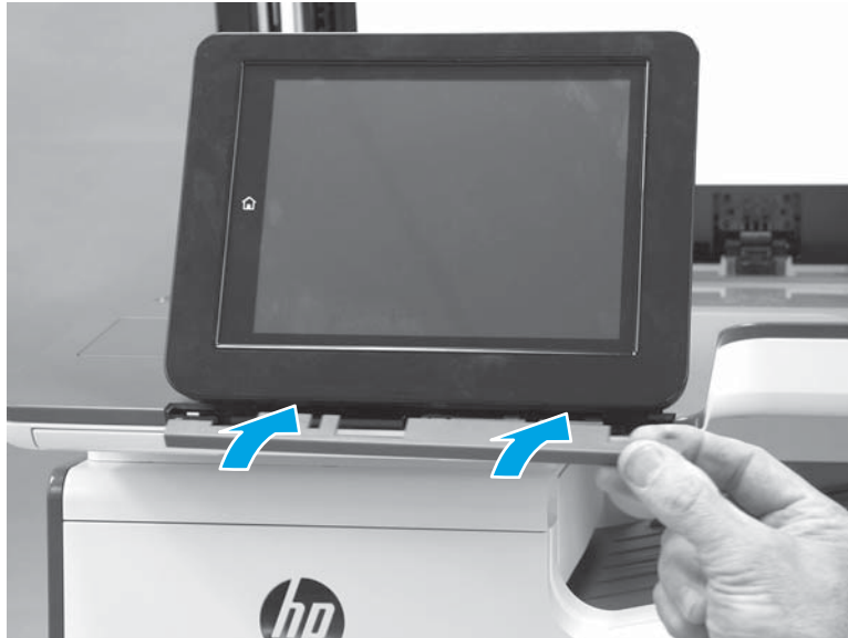
Figure 1-290 Install the cover
