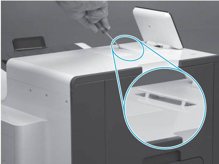
Figure 1-422 Release two tabs
