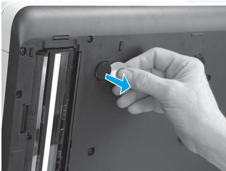
Figure 1-12 Release damaged clips
