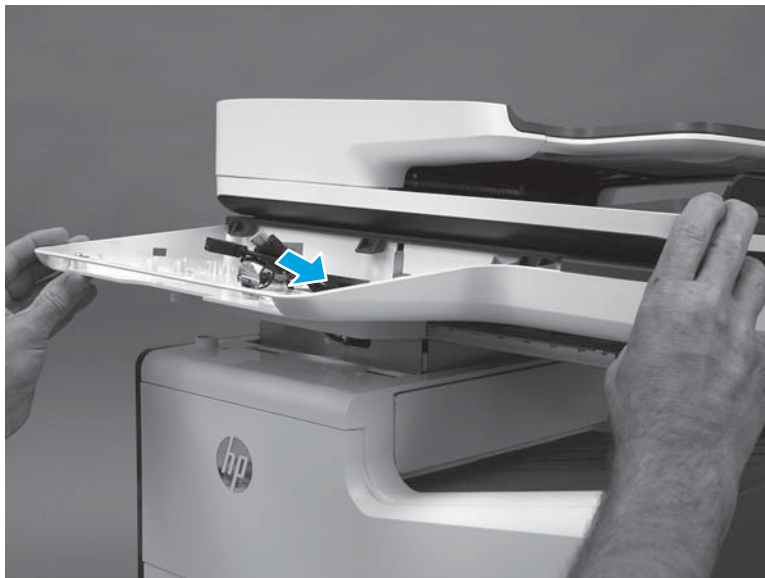
Figure 1-910 Pass the wire harnesses and cables through the opening
