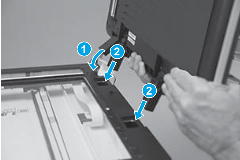
Figure 1-612 Install the document feeder
