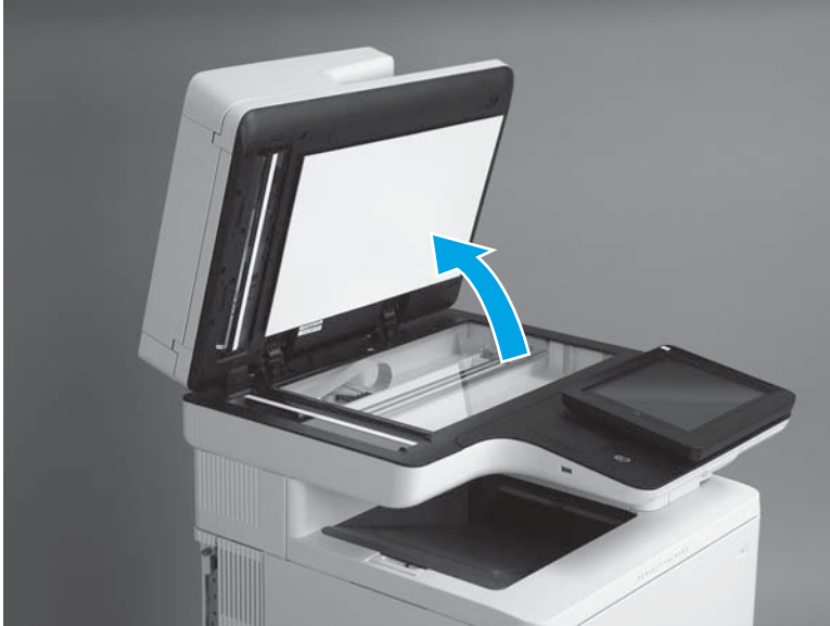
Figure 1-9 Open the document feeder
