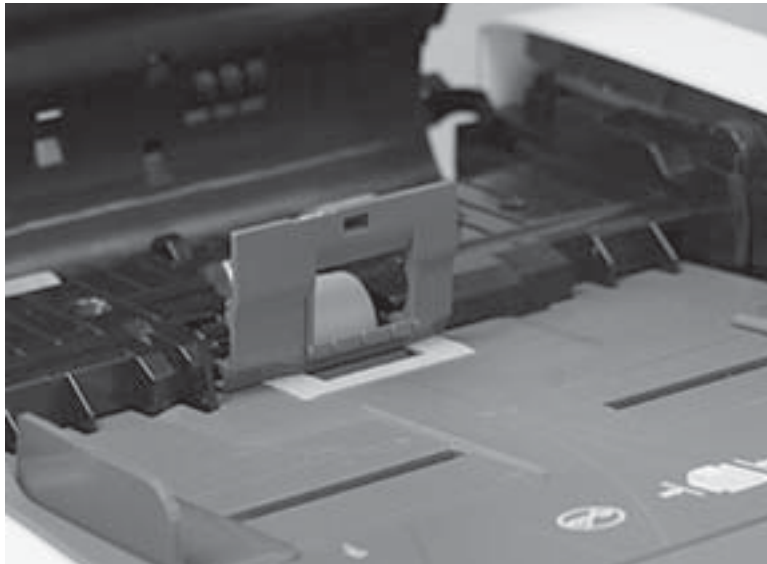
Figure 1-974 Install the roller cover
