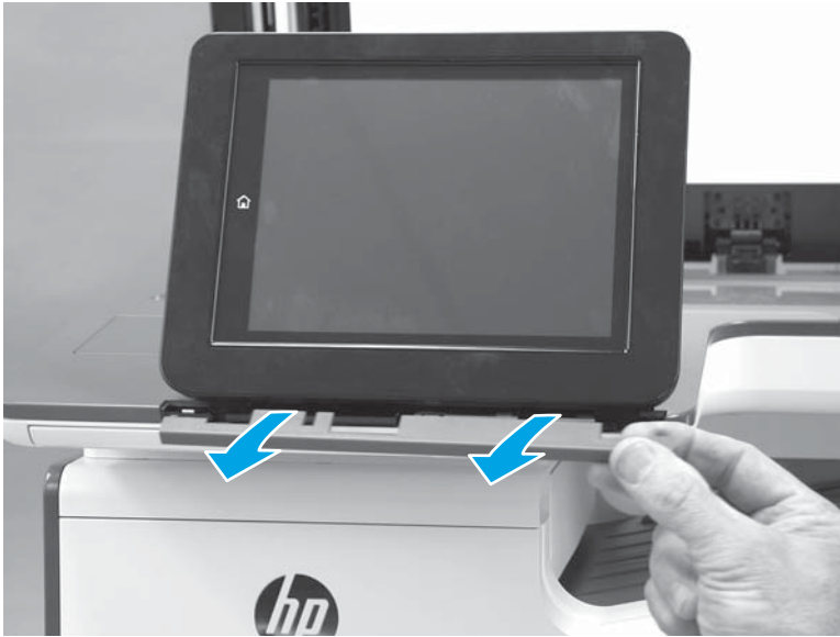
Figure 1-429 Remove the cover
