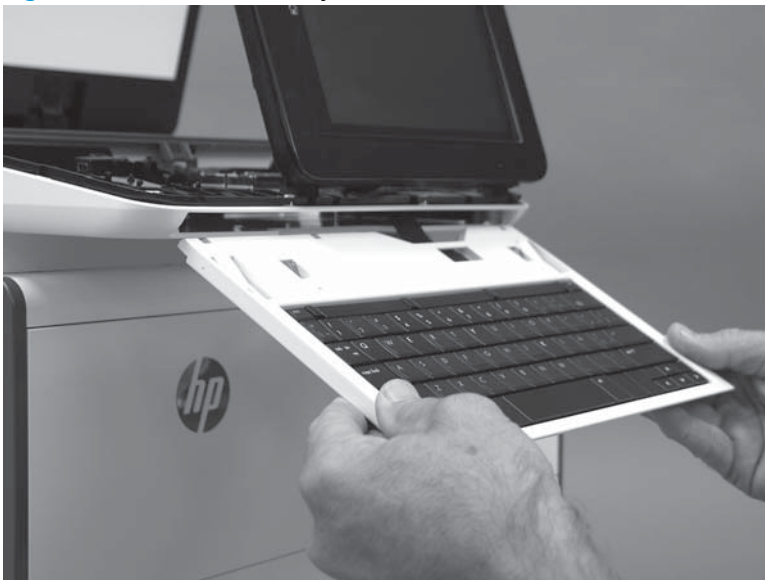
Figure 1-896 Remove the keyboard (586z)
