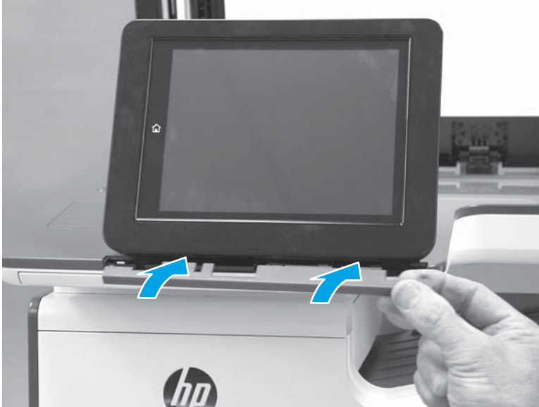
Figure 1-47 Install the cover
