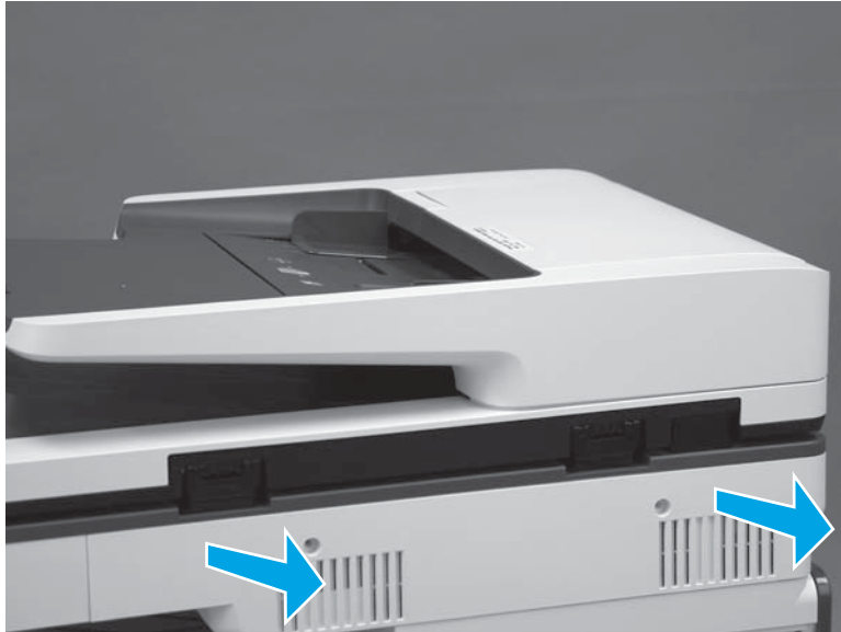
Figure 1-96 Remove the SCB cover
