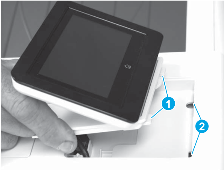
Figure 1-553 Install the control panel
