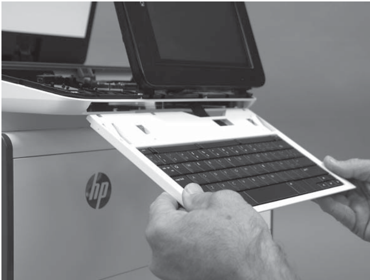
Figure 1-410 Install the keyboard (586z)
