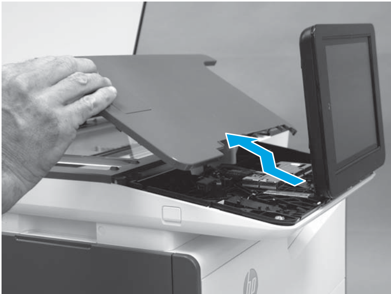
Figure 1-199 Remove the control-panel cover
