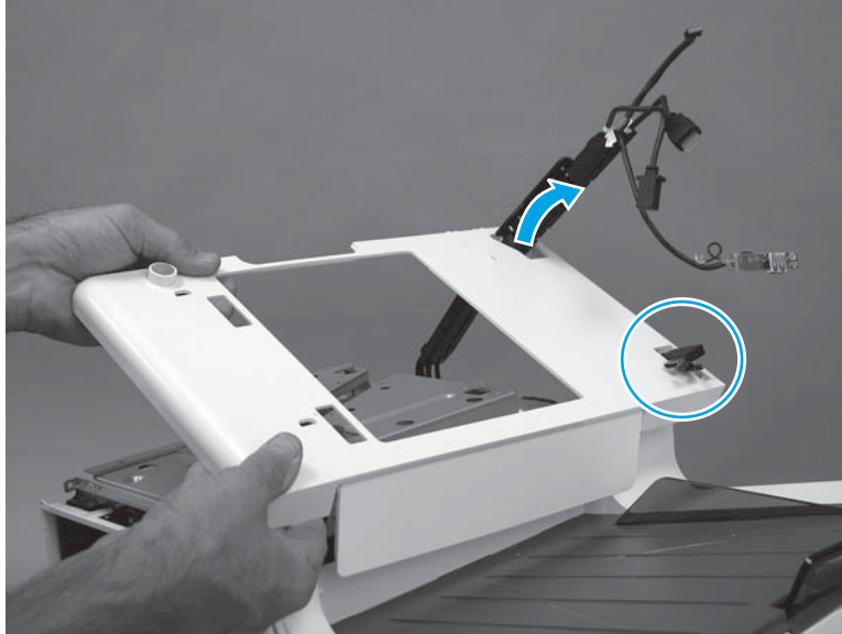
Figure 1-349 Remove the top cover (586)
