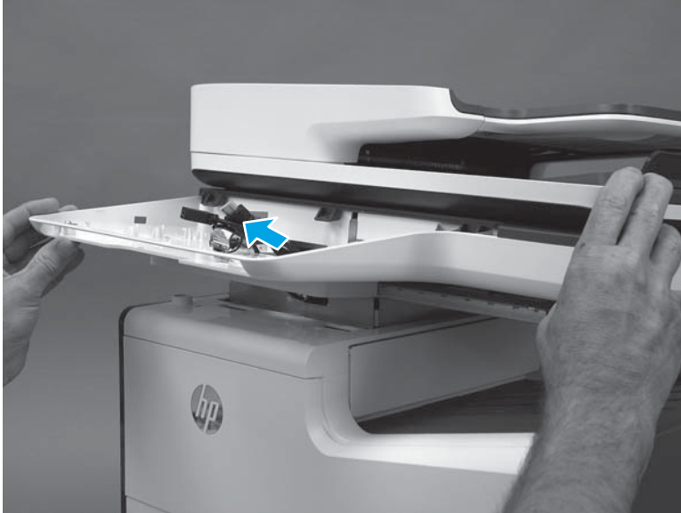
Figure 1-529 Pass the wire harnesses and cables through the opening
