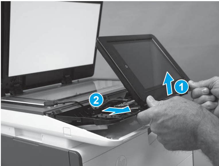
Figure 1-38 Remove the control panel
