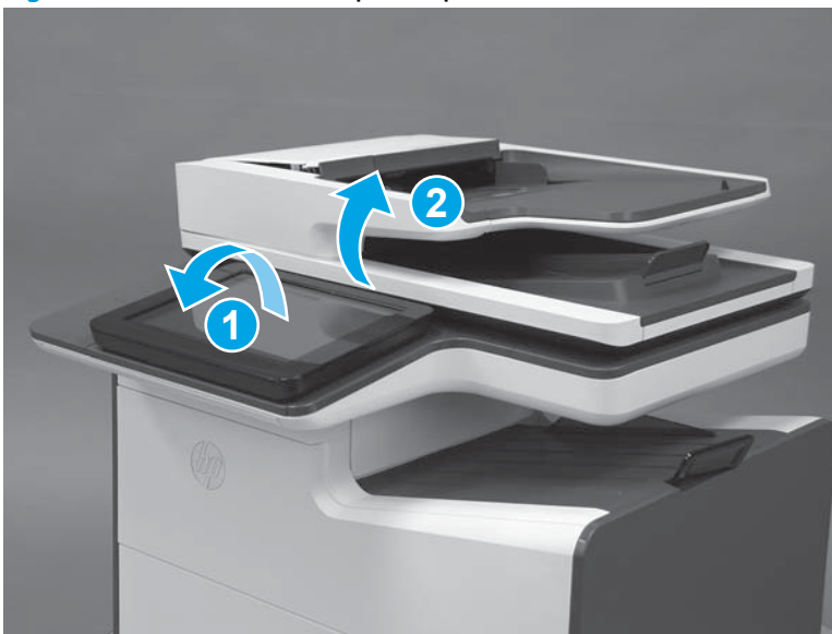
Figure 1-195 Tilt the control panel up
