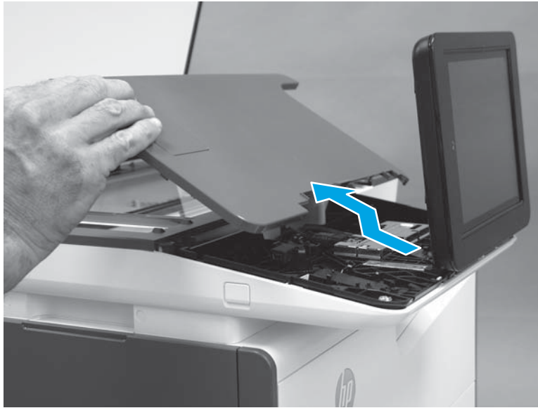
Figure 1-301 Remove the control-panel cover
