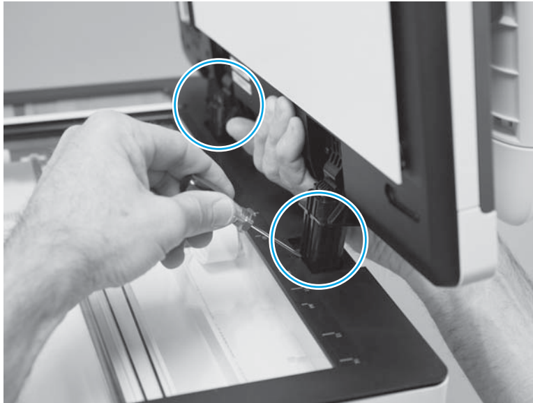
Figure 1-609 Release two tabs on the hinges
