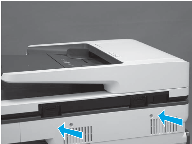
Figure 1-98 Install the SCB cover
