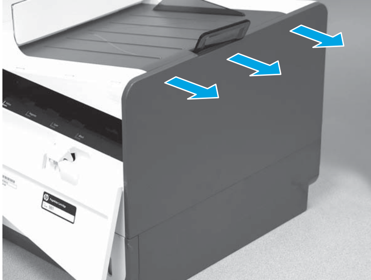
Figure 1-224 Release the right cover (outer)
