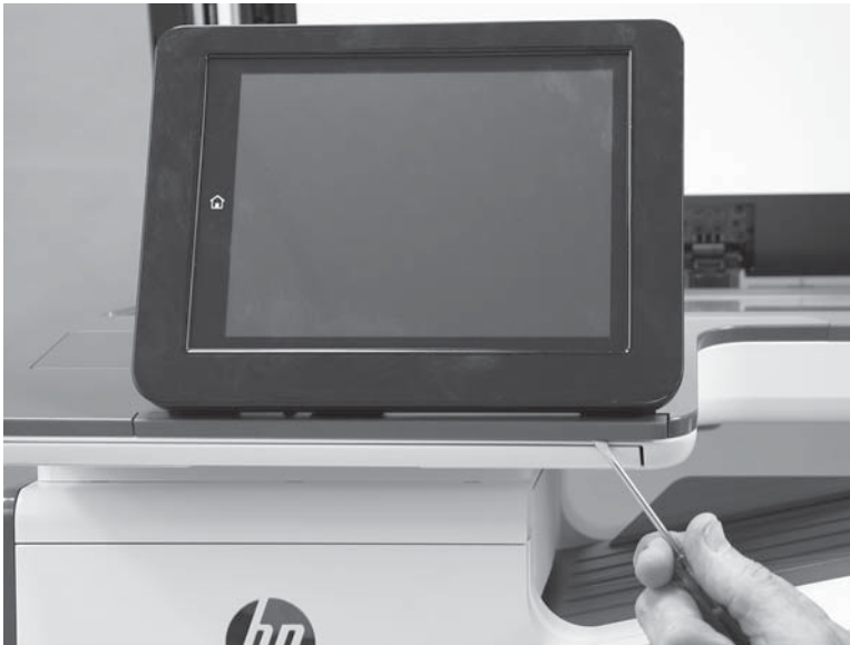
Figure 1-49 Release the small grey plastic cover
