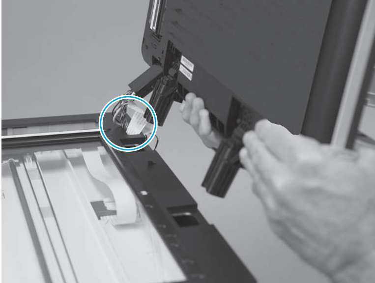
Figure 1-686 Remove the document feeder
