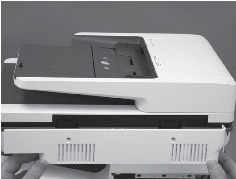
Figure 1-276 Align the tabs on the SCB cover
