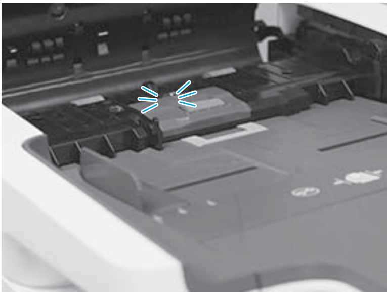
Figure 1-976 Push down on the roller cover
