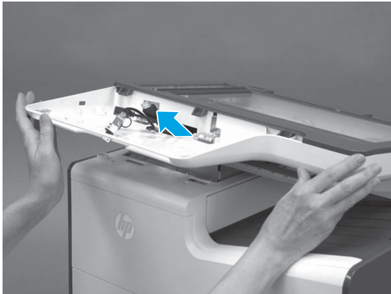
Figure 1-699 Pass the wire harnesses and cables through the opening
