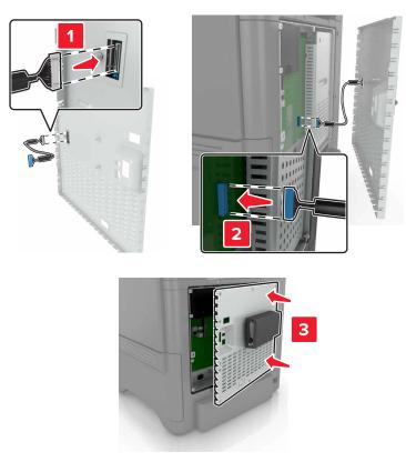
7 Reattach the controller board access cover.
