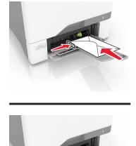
**Warning—Potential Damage:** Do not use envelopes with stamps, clasps, snaps, windows, coated linings, or self-stick adhesives.
