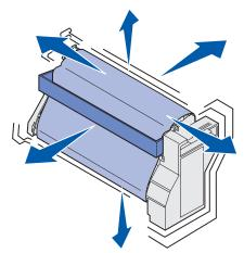
**6** Remove the cardboard shim and print cartridge detensioner.
