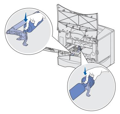
**c** Push the roller down into place at the back of the printer.
