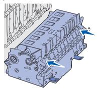
7 Slide the latches to each side and then pull up to lock the fuser in place.
