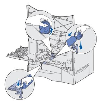
**b** Using your right hand, insert the small end of the new roller into the notched opening as shown.
