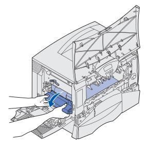
**c** Slide the unit out and place it on a clean, flat surface.
