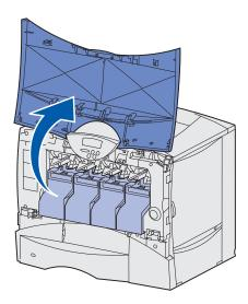
**3** Pull up slightly on the handhold. Pull the cartridge straight out and use the handle to lift the cartridge off the guides.
