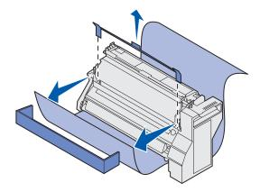
7 Remove the photoconductor drum cover and unwrap the blanket.
