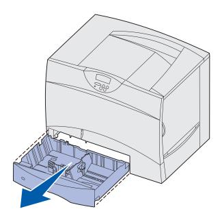
2 Squeeze the front guide lever and slide the guide to the front of the tray.
