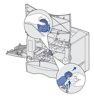
**b** While holding the rear section down, use your left hand to grab the front end of the roller.
