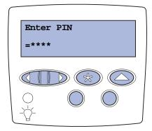
If you enter an invalid PIN, the message No Jobs Found. Retry? appears. Press **Go** to reenter the PIN, or press **Stop** to exit the Confidential Job menu.
