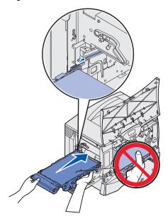
**b** Push the handle up using both hands, and gently slide in the new unit. It will drop down when correctly seated.
