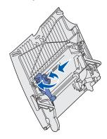
**3** Flex the specialty media back and forth to loosen the stack, and then fan the stack. Do not fold or crease the media. Straighten the edges of the stack on a level surface.
