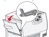
**2** Press the pick assembly release lever, and remove all media and jams.
