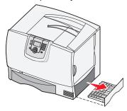
2 Remove any jams, and then reinstall the tray.
