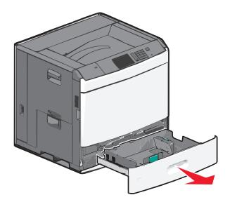
Notice the size indicators on the bottom of the tray. Use these indicators to help position the length and width guides.
