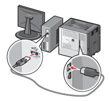
**Note:** After the printer is configured, the software will instruct you to disconnect the temporary USB cable so you can print wirelessly.
