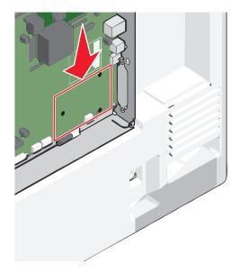
**4** Remove the printer hard disk.
