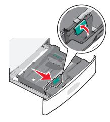
**3** Squeeze and then slide the length guide to the correct position for the paper size you are loading.
