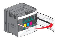
**2** Lift the green handle and pull the print cartridge. Grasp the top handle and lift the cartridge out of the machine.
