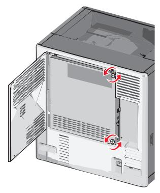
**b** Shift the metal panel to the left to disengage the hooks, then pull forward to remove it.
