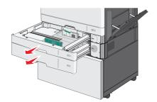
**b** Remove the screw from the 250-sheet tray.
