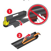
Insert the imaging unit into the printer until it *clicks* it into place.
