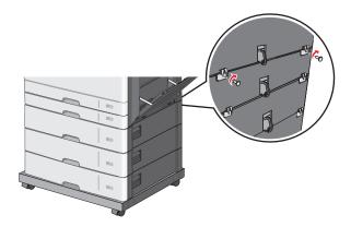
**10** Insert the bases on the slots at the sides of the caster base and secure them with screws.
