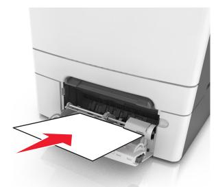
**4** Slide the paper guide until it lightly rests against the edge of the paper stack.
