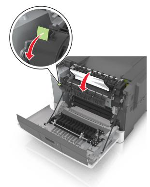
**3** Hold down the fuser cover, and then remove the jammed paper.
