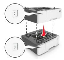
4 Align the printer with the 650-sheet duo tray, and then lower the printer into place.
