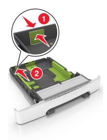
**3** Squeeze, and then slide the length guide tab to the correct position for the size of the paper being loaded.
