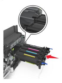
Push the blue levers down until the imaging kit is fully seated into place.
