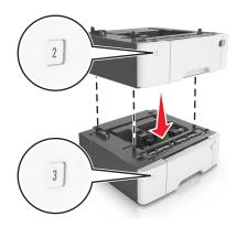
**5** Align the printer with the 650-sheet duo tray, and then lower the printer into place.
