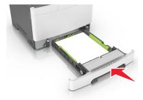
**9** From the printer control panel, set the paper size and paper type in the Paper menu to match the paper loaded in the tray.
