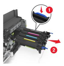
**8** Remove the used developer unit.
