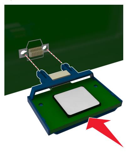
**Warning—Potential Damage:** Improper installation of the card may cause damage to the card and the controller board.
