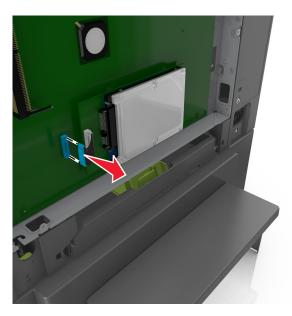
**3** Remove the printer hard disk by pulling it away from the controller board.
