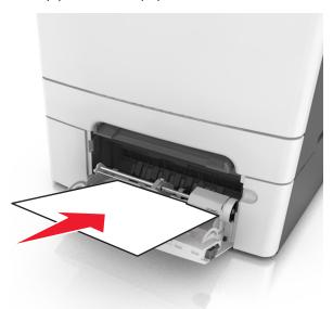
Slide the paper guide until it rests lightly against the edge of the paper stack.
