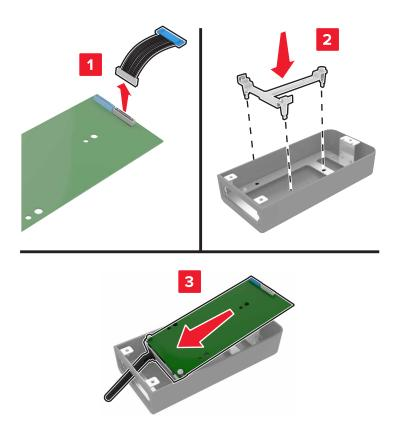
Attach the housing to the controller board access cover.
