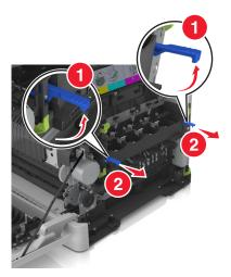
7 Press down the blue lever, and then grasp the green handles on the sides to pull out the imaging kit.
