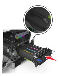
**13** Gently but firmly push the blue levers down until the imaging kit fits into place.
