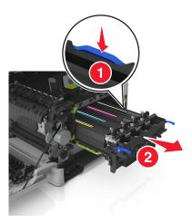
**8** Remove the used developer unit.
