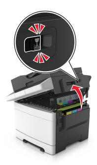
**2** Remove the toner cartridge by lifting the handle, and then gently pulling it away from the imaging kit.
