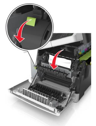
**c** If there is a jammed paper in the fuser, then hold down the fuser cover, and then remove the paper.
