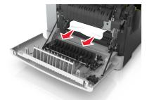
**b** Pull the green lever to open the fuser cover.
