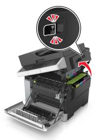
**3** Pull the green lever to open the fuser cover.
