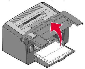
**Note:** It may be necessary to remove the toner cartridge and place it on a flat, clean surface to reach print media lodged behind it. Replace the toner cartridge when the print media has been located and removed.
