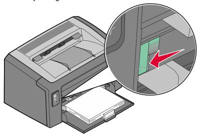
**5** Pull the front door up until it *clicks* into an open position, and remove any lodged print media.
