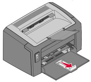
**Note:** To decrease width, push in on the left guide. To increase width, squeeze the tab attached to the right guide, and slide it to the right.
