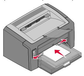
Note: Do not force print media into the feeder. Forcing print media causes jams.
