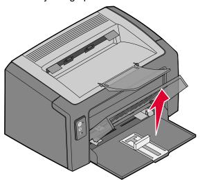
2 Adjust the slide and attached backstop to the length of the selected print media.
