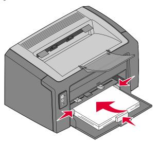
**Note:** Load letterhead paper with the design side facing up and the top edge of the sheet feeding into the printer first. Load envelopes with the flap side down and the return address first. The stamp area will feed through last.
