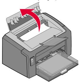
**CAUTION:** The fuser may be hot. To avoid personal injury, use caution when opening the top door to remove a jam from the fuser area.
