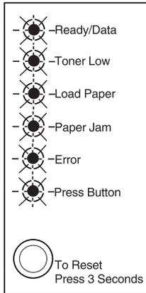
Press and release the operator panel button to display the secondary service error code.
