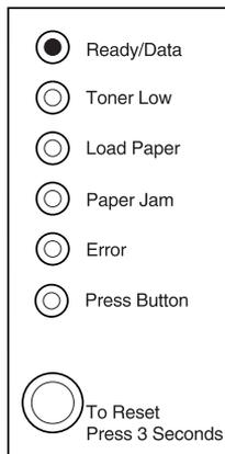
Ready indicates the printer is ready to receive and process data from the host system.
