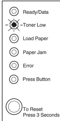
Once the error code is displayed, and if the operator panel button is pushed again, the operator panel displays the service error indication (all six indicator lights blinking). Continual pressing of the button causes the lights to repeat in the following order:
