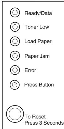
Depending on the light sequence, briefly (approximately one second) push the operator panel button to restart the printer, display an error code, or activate other printer functions.
