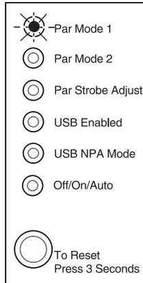
For the solid lights, the lit Par Enabled (Ready) light means the panel is presently showing the value for the menu item Parallel Port Enabled. The off/on/auto (Press Button) light displays the value of the current setting: off, on, or auto. (For this example, Parallel Port Enabled is off.) The value list for the menu item Parallel Enabled is off, on, and auto.
