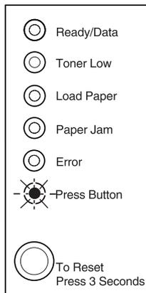
**Fuser failure–thermistor open error code**
