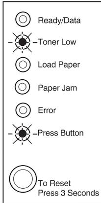
Once the subcode is displayed, if the operator panel button is pushed again, all six indicator lights blink. Continual pressing of the operator panel button causes the lights to repeat in the following order:
