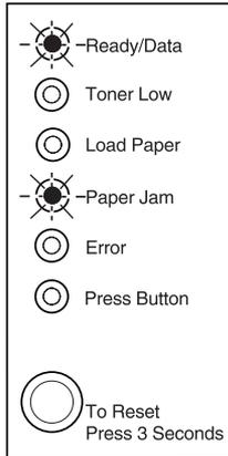
Once the error code is displayed, if the operator panel button is pushed again, the operator panel will display the service error indication (all six indicator lights blinking). Continual pressing of the operator panel button causes the lights to repeat in the following order:
