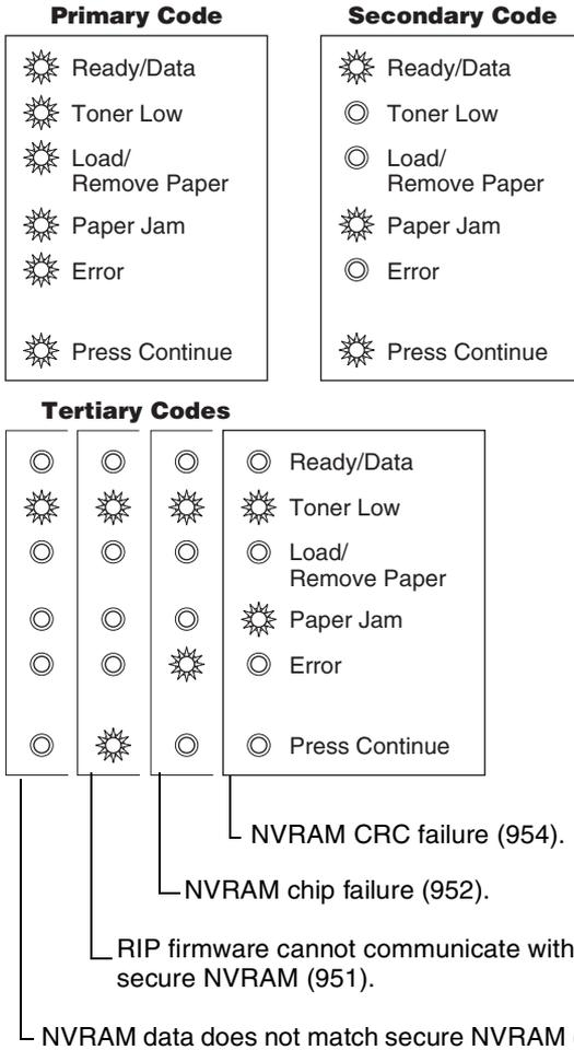
**Note:** NVRAM is on the operator panel printed circuit board (PCB) while secure NVRAM is on the controller PCB. Check margin alignments after replacing the operator panel assembly. See **“Printhead assembly ” on page 4-2** (steps 1 through 11) for more information. If margin errors are unacceptable, corrections can only be made through software. Contact the next level of support or Lexmark at 1–800–539–6275.
