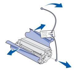
Warning: Do not touch the photoconductor drum on the bottom of the print cartridge.
