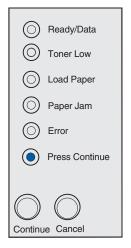
The printer is not ready to receive or process data, or the printer ports are offline. In addition, the toner in the print cartridge is getting low.
