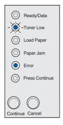
The print cartridge you are using was not designed for your printer.
