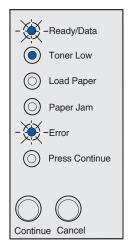
The printer prompts you to load a single sheet of media in the manual feed.
