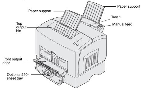
An exit output bin on top of the printer holds up to 100 sheets. The single-sheet front output door provides a straight-through paper path for special media, such as transparencies, envelopes, labels, card stock or index cards, reducing curling and potential paper jams.
