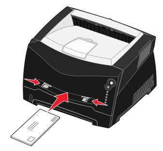
Warning: Do not force the print media into the feeder. Forcing the media causes jams.
