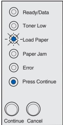
When the Load Paper light is blinking and the Press Continue light is on solid, the printer prompts you to load a single sheet of media.
