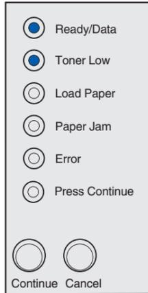
When the Ready/Data light and Toner Low light are on solid, the printer alerts you that the toner is getting low. To use the remaining toner, remove the print cartridge, gently shake it back and forth, and reinsert it. When the print fades or is unsatisfactory, replace the print cartridge.
