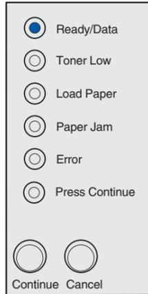
When the Ready/Data light is on solid, the printer is ready to receive and process data.
