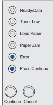
When the Error light and Press Continue lights are on solid, a secondary error has occurred.
