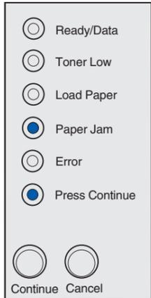
When the Paper Jam light and the Press Continue lights are on solid, the printer detects a jam.
