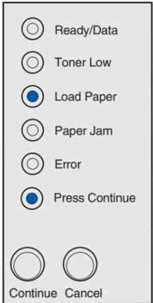
When the Load Paper light and the Press Continue lights are on solid, the printer is out of media, or the media did not feed properly.
