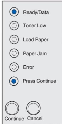
When the Ready/Data light and Press Continue lights are on solid, the printer is waiting for additional data.
