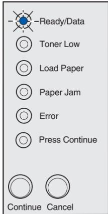
When the Ready/Data light is blinking, the printer is busy receiving or processing data.
