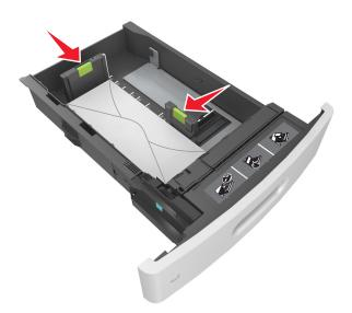
• Make sure the paper is below the solid line, which is the maximum paper fill indicator.
