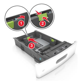
**3** Unlock the length guide, and then squeeze and slide the guide to the correct position for the size of the paper being loaded.
