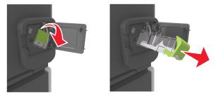
**3** Open the staple guard, and then remove the loose staples.
