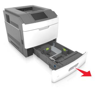
**Note:** Use the paper size indicators at the bottom of the tray to help position the guides.
