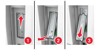
**5** Align the posts of the plastic bracket with the holes on the controller board cage, and then press the plastic bracket on the controller board cage until it *clicks* into place. Make sure the cables are neatly tucked under the plastic bracket.
