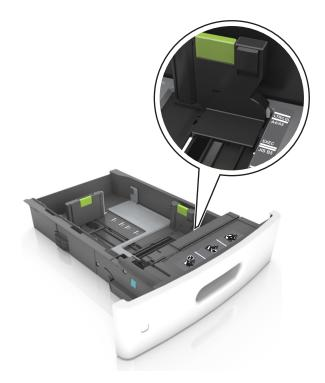
**3** Unlock the length guide, and then squeeze and slide the guide to the correct position for the size of the paper being loaded.
