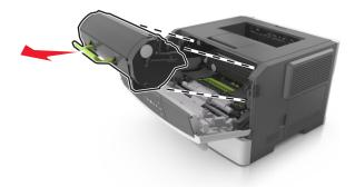
**3** Lift the green handle, and then pull the imaging unit out of the printer.
