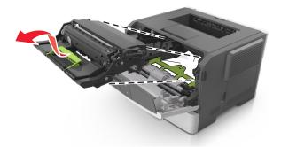
**Warning—Potential Damage:** Do not expose the imaging unit to direct light for more than 10 minutes. Extended exposure to light may cause print quality problems.
