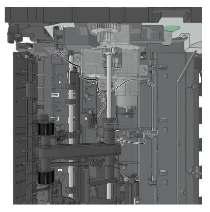
**c** Secure the cable at the pick/lift motor gearbox using cable ties. Cut off any excess cable tie.
