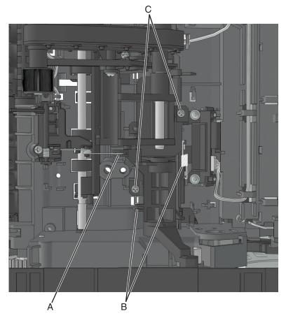
Below are the cam release and bracket.
