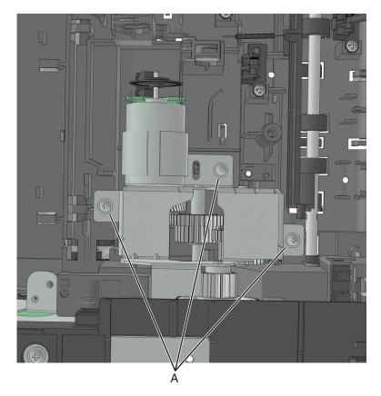
**9** Disconnect the cable from the pick/lift motor gearbox.
