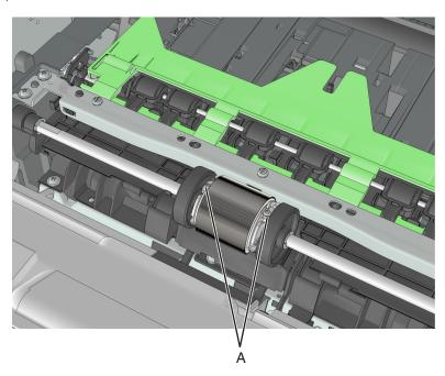
**3** Pull the MPF pick roller outward to remove.
