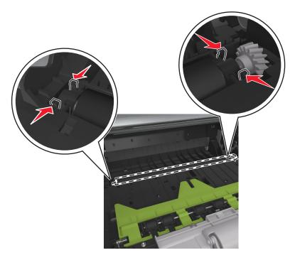
**2** Lift to remove the transfer roll.
