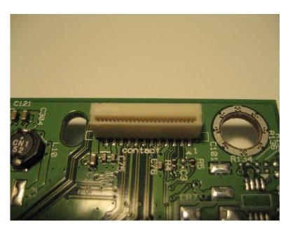
**2** Insert the cable squarely into the connector.
