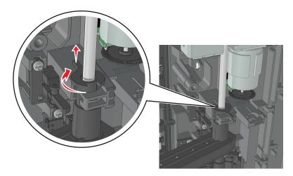
**9** Remove the ACM assembly along with its shaft.
