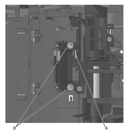
**9** Disconnect the cable from the sensor.
