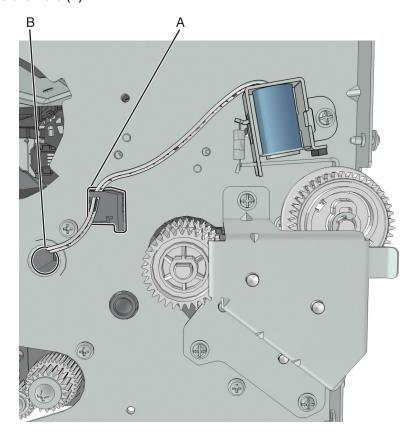
**d** Route the cable using the new path.
