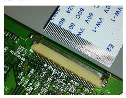
**3** Rotate the locking actuator to the locked position. The cable should not move while this step is performed. If the cable moves, open the actuator, reposition the cable, and then close the actuator to the down position.
