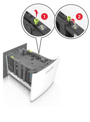
**b** If the A5 length guide is still attached to the length guide, then remove it from its place. If the A5 length guide is not attached, then proceed to step d.
