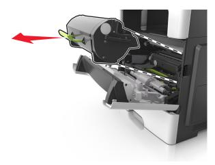
**3** Lift the green handle, and then pull the imaging unit out of the printer.
