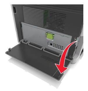
**2** Open the controller board shield using the green handle.
