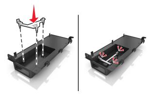
Slide and push the ISP solution into the plastic bracket.
