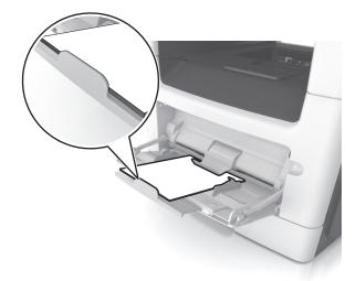
• Load letterhead faceup with the top edge entering the printer first. For two-sided (duplex) printing, load letterhead facedown with the bottom edge entering the printer first.
