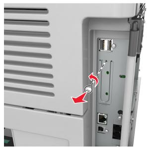
**b** Lift the metal cover, and then pull it out completely.
