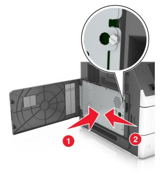
**6** Tighten the screws on the shield.
