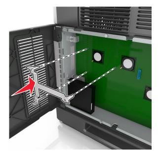
**Note:** Make sure that the plastic bracket has latched completely, and that the plastic bracket is seated firmly on the cage.
