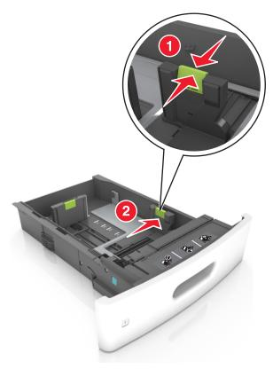
Note: Use the paper size indicators at the bottom of the tray to help position the guides.
