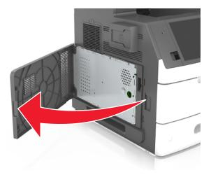
**2** Using a screwdriver, loosen the screws on the controller board shield.
