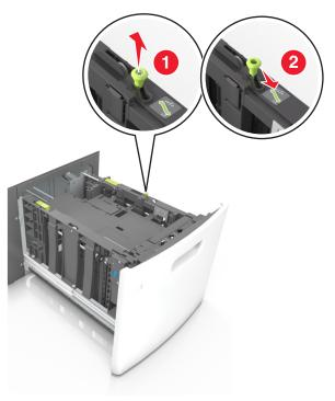
**b** Squeeze, and then slide the length guide to the position for A5 until it *clicks* into place.
