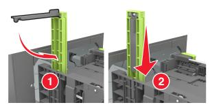
**d** Squeeze, and then slide the length guide to the correct position for the paper size you are loading.
