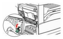
**Note:** If the jam does not move immediately, stop pulling. Push down and pull the green lever to make it easier to remove the jam. Make sure all paper fragments are removed.
