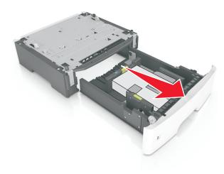
**4** Remove any packing material from inside the tray.
