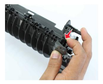
If necessary, remove the bushing (B) from the redrive assembly.
