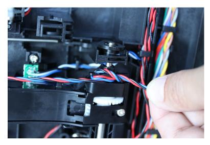
**h** Route the cable using the new path, and secure it with a cable tie (A).
