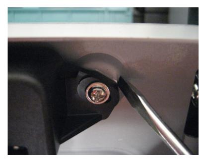
**9** Remove the three screws (B) securing the LSU.
