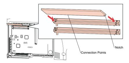
3 Insert the memory option all the way into the connector at a 45° angle, and rotate it down until it snaps into place.
