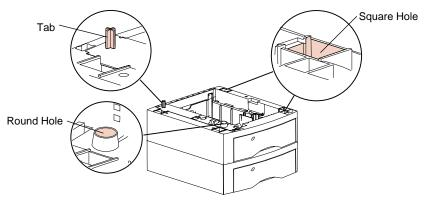
**Note:** When you lift the duplex option for placement, remember it contains the removable duplex front access cover. Lift the duplex option from the bottom at opposite corners. Keep the duplex option level as you move it so the duplex front access cover does not fall out.
