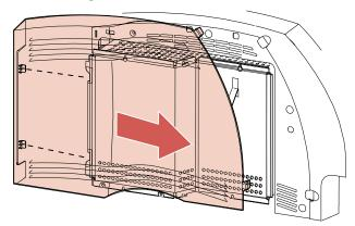
Close the side door, pressing on the side door latches to snap it into place.
