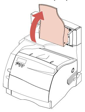
**2** Pull the tray straight out toward you to remove the upper tabs from the output expander slots.
