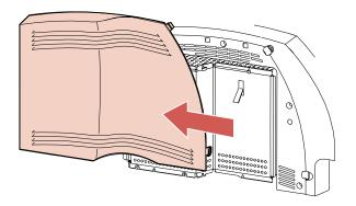
5 Loosen the six screws on the shield. Do not remove the screws.
