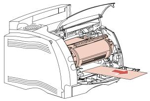
**Note:** You may have to remove the print cartridge before you can pull the envelope out.
