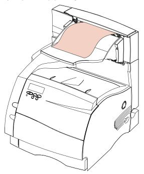
Locate and push the output expander rear door latches in toward the center.
