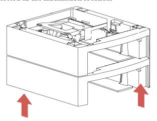
5 Locate the following parts on the top surface of the upper support unit: the tab, the round hole, and the four square holes. The bottom surface of the printer has matching holes or feet that accommodate the tab, round hole, and four square holes.
