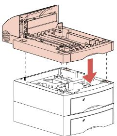
**8** Notice the following parts on the duplex option: the tab, the round hole, and the four square holes. These are exactly like the same parts on an optional or standard paper drawer. The printer has matching holes on its bottom surface that align with these parts.
