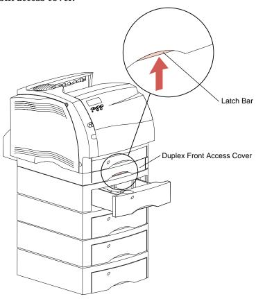
**3** Push the latch bar up and pull the duplex front access cover straight out from the duplex option.
