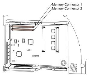
Before you install a memory option, follow the steps under "Accessing the Printer System Board" on page 293.
