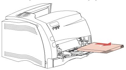
**2** Push the metal bar straight back to collapse the multipurpose feeder to its short-length position.
