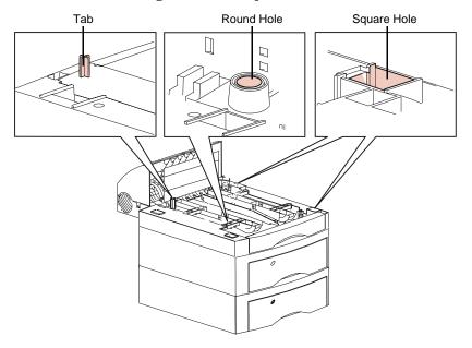
**9** Lift the printer by the hand grips or ask someone to help you lift it and lower it onto the duplex option. Be sure the edges of the printer and the duplex option are aligned so that all the parts fit.
