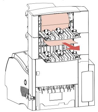
**5** Close both of the output expander rear doors. Make sure all rear door latches are closed.
