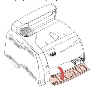
**3** Grasp the lower right corner of the envelope feeder connector door and pull it up. The connector is exposed.
