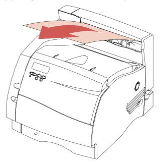
Open the upper front door to release the fuser rollers.
