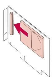
**2** Push the hard disk securely into the connector.
