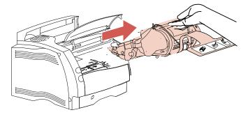
5 Pull on each end of the plastic, V-shaped piece and then pull the packaging material straight out. Discard all packaging material: the V-shaped piece, the foam, and the paper connected to the foam.
