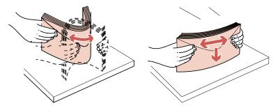
**Note:** When you load envelopes, do not exceed the maximum stack height of 64.7 mm (2.55 in.). The envelope feeder holds a maximum of 85 envelopes (75 g/m $^2$ , 20 lb bond).
