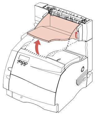
Note: At this point, you may attach another output expander to the output expander you just installed. To do this, complete step 3 on page 284 again, but install the mounting brackets of the second expander into the mounting slots on the first output expander you installed. Complete step 4 on page 286 to step 6 on page 287 to install the second output expander tray.
