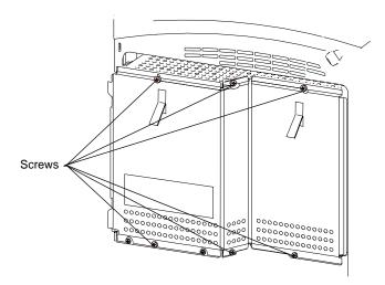
6 Grasp the tabs and slide the shield up until the top three screws fit into the three keyholes on the shield. Holding the shield by the tabs, lift it off.
