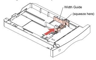
Note: Before you put paper in the tray, adjust the tray size for your paper. This example shows how to adjust for letter size paper (LTR). Notice the *paper size indicators* printed on the top left surface of the tray. These abbreviations indicate the paper sizes. The paper size indicators help you in the placement of the length guide.
