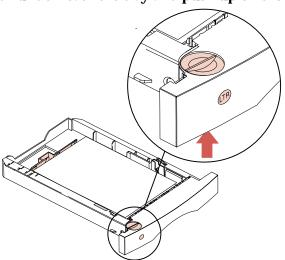
**3 Pull the knob out of the tray.** Notice the label on the lower portion of the knob.
