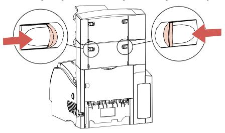
**2** Open the output expander rear door for the output expander installed above.
