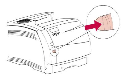
The multipurpose feeder door drops open and stops in place.
