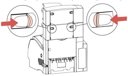
**3** Open the output expander rear door for the one installed above. When complete, two output expander rear doors are open.
