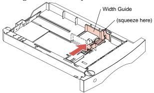
**Note:** Before you put paper in the tray, adjust the tray size for your paper. This example shows how to adjust for letter size paper (LTR). Notice the *paper size indicators* printed on the top left surface of the tray. These abbreviations indicate the paper sizes. The paper size indicators help you in the placement of the length guide.
