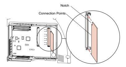
3 Press the flash memory option down toward the system board until it snaps into place. Make sure both metal clips on the connector are fastened and the two pins on the connector are pushed through the holes in the option.
