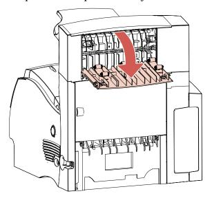
**3** Loosen the paper if it is caught in feeder rollers. Then, pull the paper straight out.
