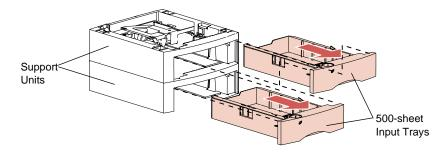
3 Remove all packing material and tape from the trays.
