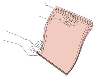
Notice the print materials stack height limiter on the left side of the multipurpose feeder. Use it as a guide for stack height when loading print materials.
