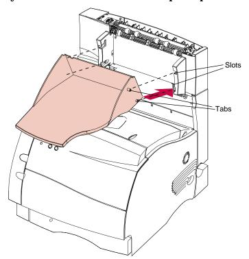
6 Rotate the output expander tray upward from the front and slide the upper tabs on the tray into the upper slots on the output expander. The tabs click in place.
