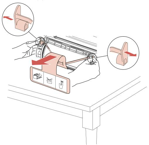
6 Reinstall the print cartridge. Align the side slides on the print cartridge with the slots on the print cartridge cradle. Use the colored arrows inside the printer for placement.
