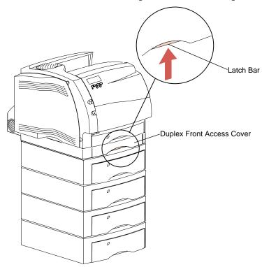
**2** Pull the duplex front access cover straight out from the duplex option. The edge of the paper is visible.
