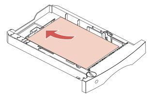
When the paper is loaded into the tray, the paper is stacked at an angle. The paper tray wall at the front of the tray is angled as this cross-section of the tray illustrates. If you readjust the length guide lever once the paper is in the tray, do not push it too far. Pushing the length guide too far causes the paper to move up along this angled wall and jam.
