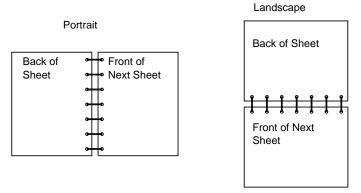
Short edge binding means all pages are attached along the short edge of the page (the top edge of a portrait printed page and the left edge of a landscape printed page). For example, the pages in a stenographer's pad are bound along the short edge.
