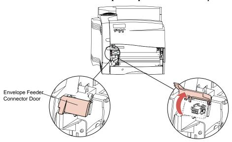
4 Align the tabs on the envelope feeder with the slots on both sides of the printer and gently push the envelope feeder into the opening until it snaps into place. The envelope feeder tilts downward at a slight angle if it is installed properly.
