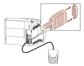
Aim the computer infrared port at the infrared port on the front of the infrared adapter. Refer to the documentation that came with your computer for information about your computer infrared port.
