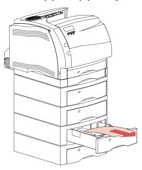
If the paper is between two trays, when you pull the tray out of the support unit, the top edge of the paper springs out toward you. Pull the paper straight up, and then out.
