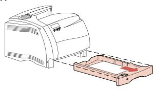
2 Squeeze the width guide lever and slide the width guide to the far right side of the tray.
