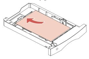
When the paper is loaded into the tray, the paper is stacked at an angle. The paper tray wall at the front of the tray is angled as this cross-section of the tray illustrates. If you readjust the length guide lever once the paper is in the tray, do not push it too far. Pushing the length guide lever too far causes the paper to move up along this angled wall and jam.
