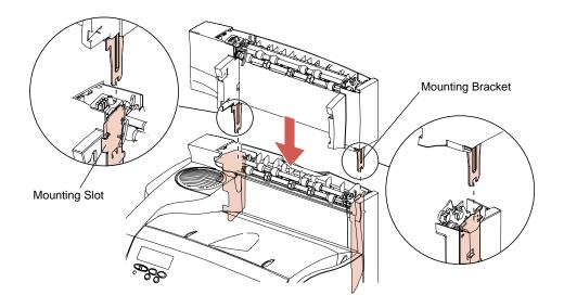
**Note:** Make sure the output expander is connected securely.
