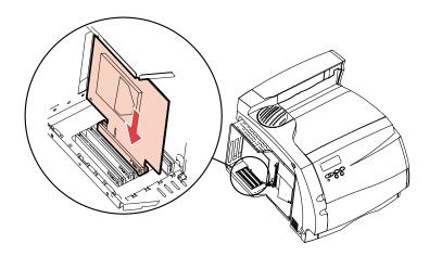
**6** Push in the card firmly until it is completely inserted into the system board connector. The two connectors should fit snugly together.
