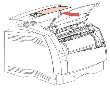
Note: Usually with a jam located in this area, there is another jam behind the rear door of the printer. See "Before Reaching the Standard Output Bin or Entering to the Duplex Option" on page 214 for instructions on how to remove this type of jam.
