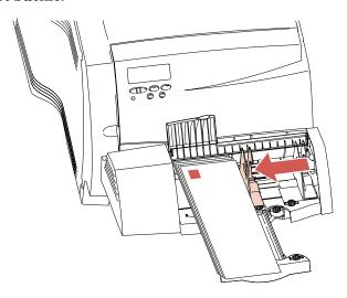
**9** Rotate the envelope weight back toward you and lower it to the stack.
