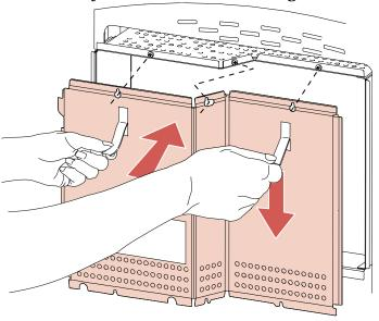
Holding the side door slightly to the left of the printer, slide the door to the right into the notches on the shield. The door hinges fit into the notches.
