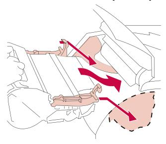
**7 Guide the print cartridge down as it drops into place.** The cartridge snaps into place.
