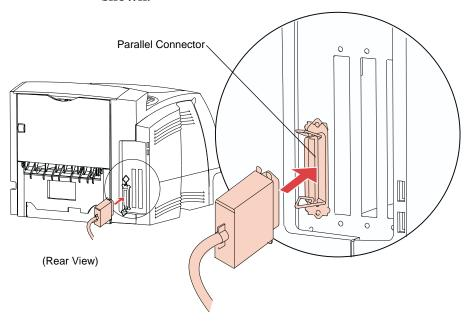
**2** Push the clips at each end of the connector into the notches on the parallel cable. The clips snap when pushed into the notches.
