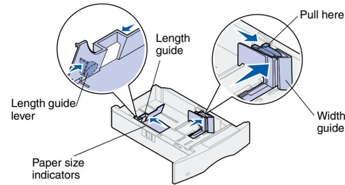
Complete these instructions to load print materials into any of the standard or optional trays. All paper trays are loaded the same way.
