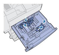
3 Place the print media against the front left corner of the tray. Labels on the tray indicate paper size and orientation.
