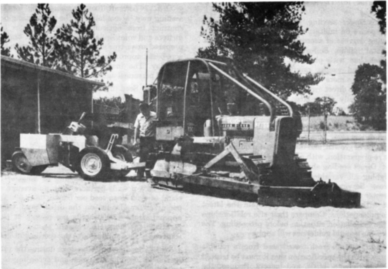
Figure 4-5. V-pusher equipped tractor with heavy duty tree planter attached.
