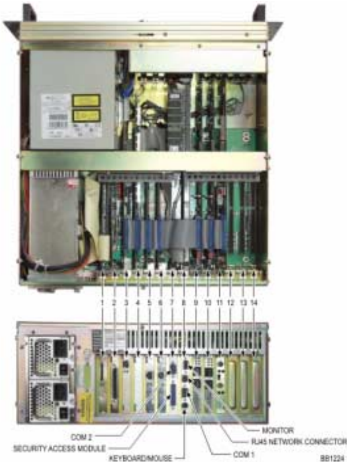
Figure 10: 1400/1400SR Card Layout Example
