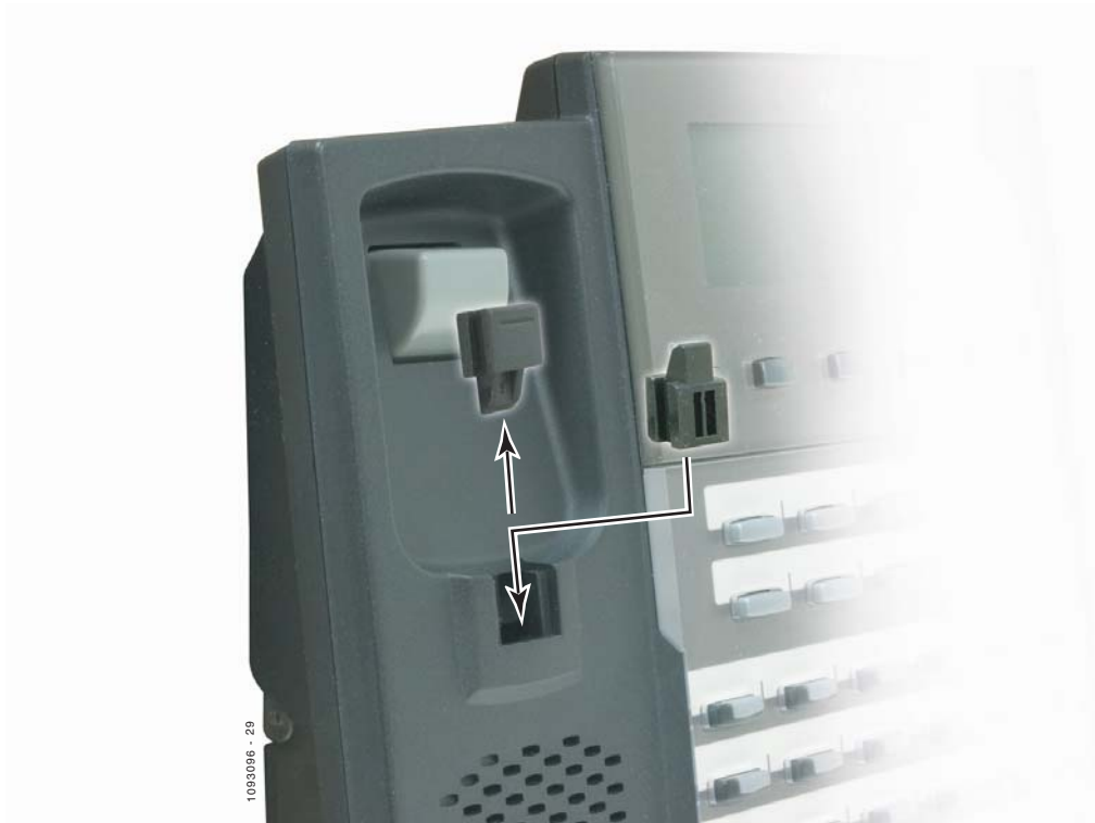
Figure 36: Reversing the Handset Hanger
