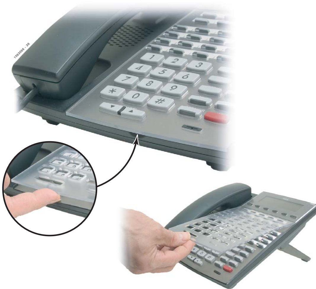
Figure 21: Removing the Telephone Faceplate
