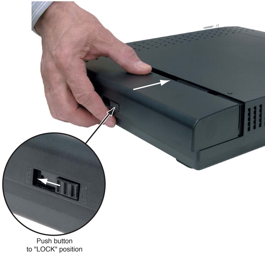
Figure 25: Reinstalling the Cover
