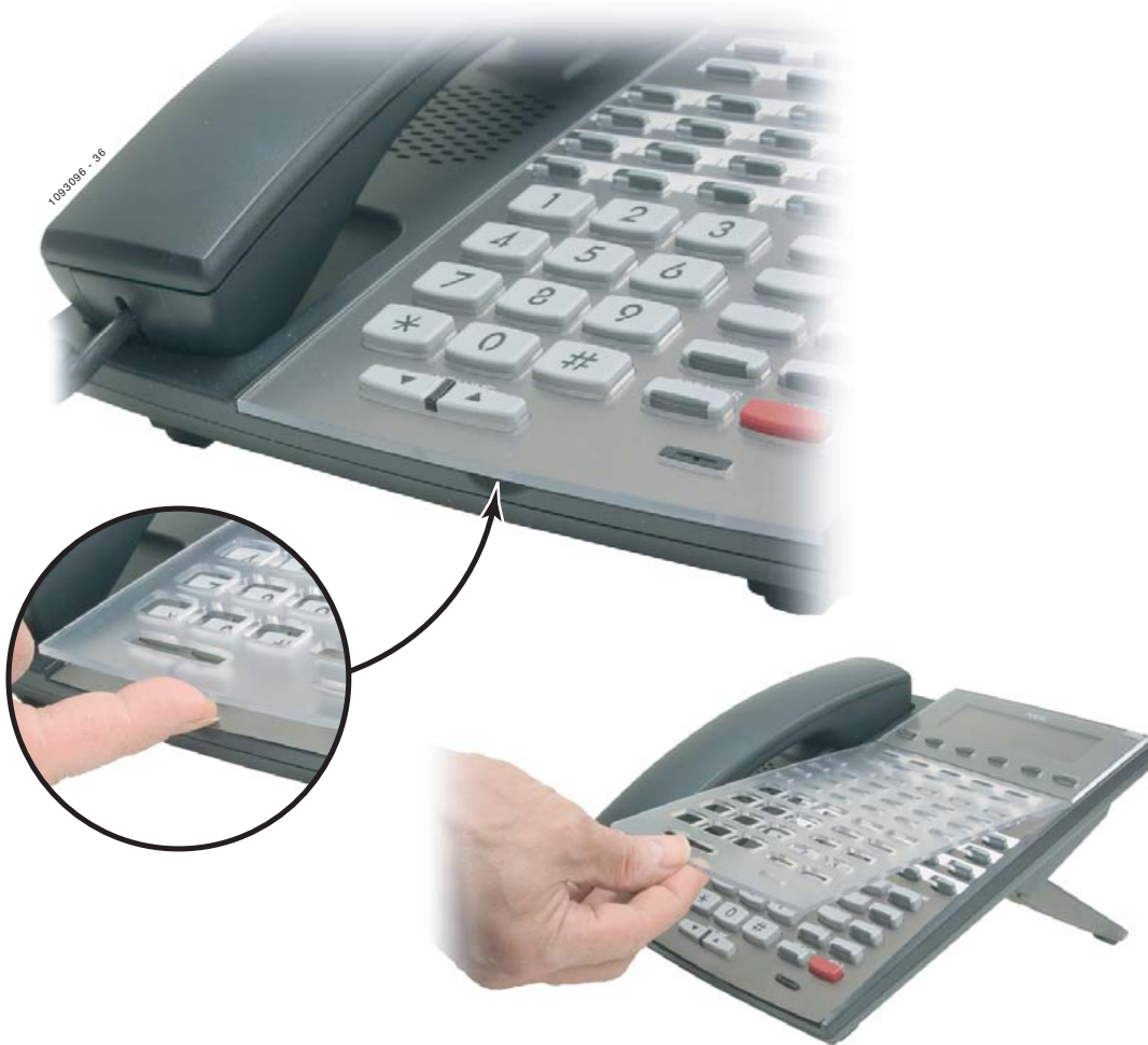
Figure 30: Removing the Telephone Faceplate
