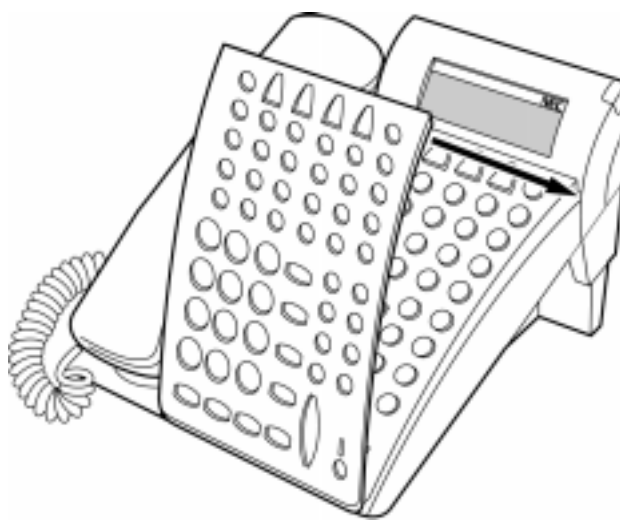
Figure 4-45 Installing Plastic Panel on a Telephone
