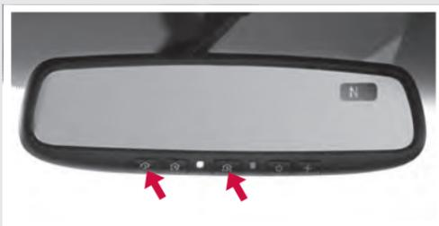
**NOTE: Once you have pressed and released the program button on the garage door opener's motor and the “training light” is lit, you have 30 seconds in which to perform step 7. Use the help of a second person for convenience to assist when performing this step.**
