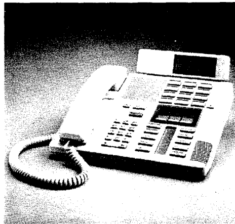
The Busy Lamp Field attached to an M7310 telephone
