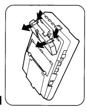
Rotate the stand ½ turn so that the arrow on the stand shows UP for WALL.
