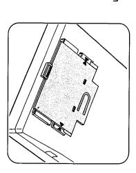
Push the two shaded arrow "A". then slide down toward under the slide rails and portions slightly and insert the edges of the holder
