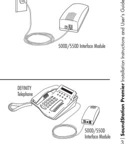
(If the connector does not fit you will need one of the optional cables as a replacement for your phone cable. This cable has a smaller connector on one end, so try it both ways.)
