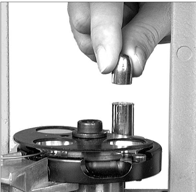
Figure 36 – Placing a bullet on the cartridge case at Station #3.
