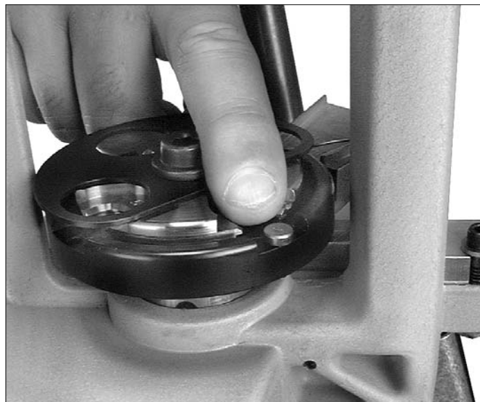
Figure 21 – Installing a brass locator button at Station #2.
