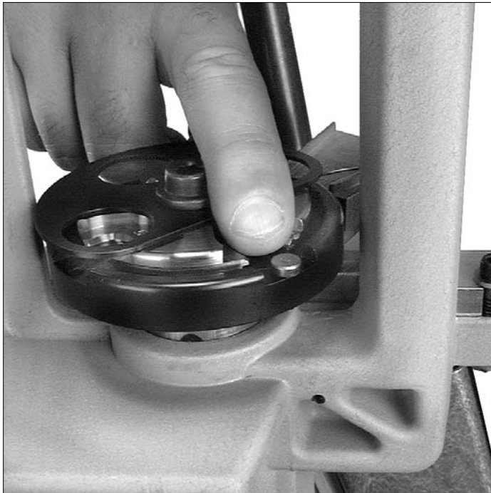
Figure 32 – Installing a brass locator button in Station #2.
