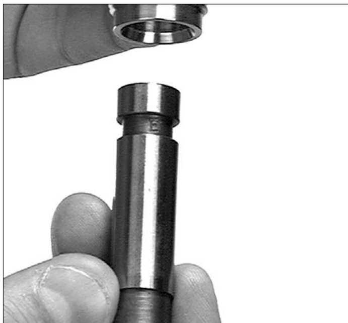
Figure 26 – The groove in the pistol powder funnel.
