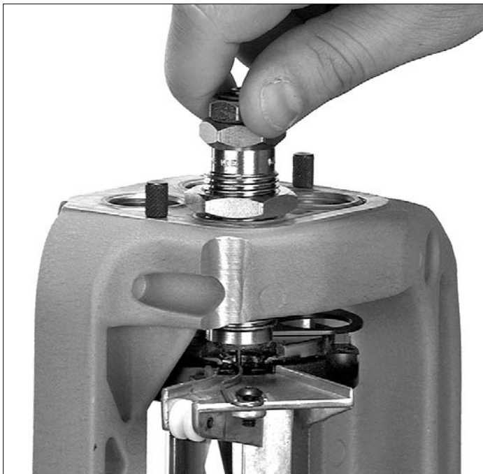
Figure 23 – Installing a sizing/decapping die in Station #1.
