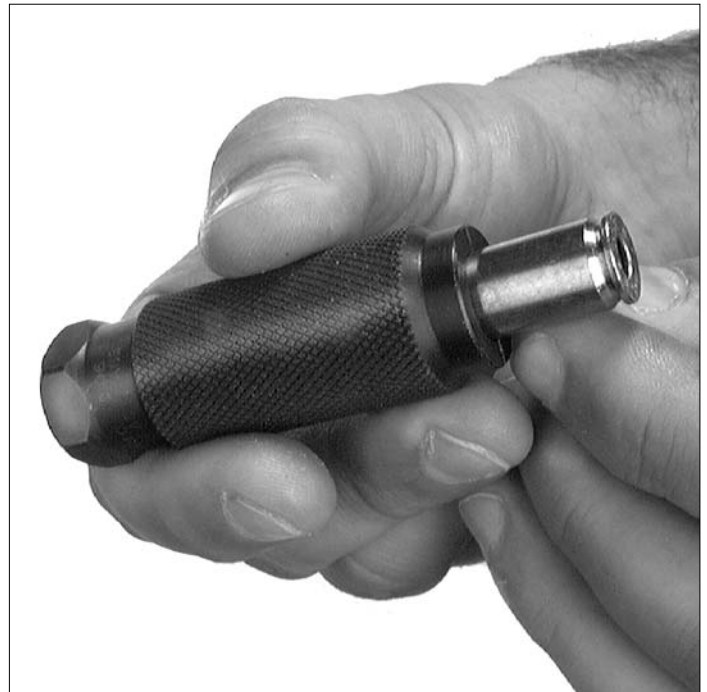
Figure 14 – Inserting a case in a case gage.
