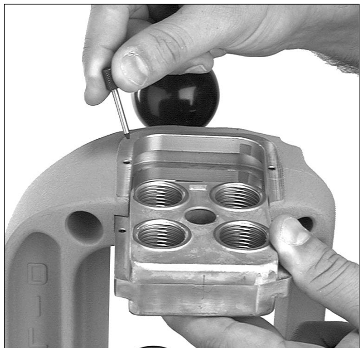
Figure 10 – Removing the toolhead.
