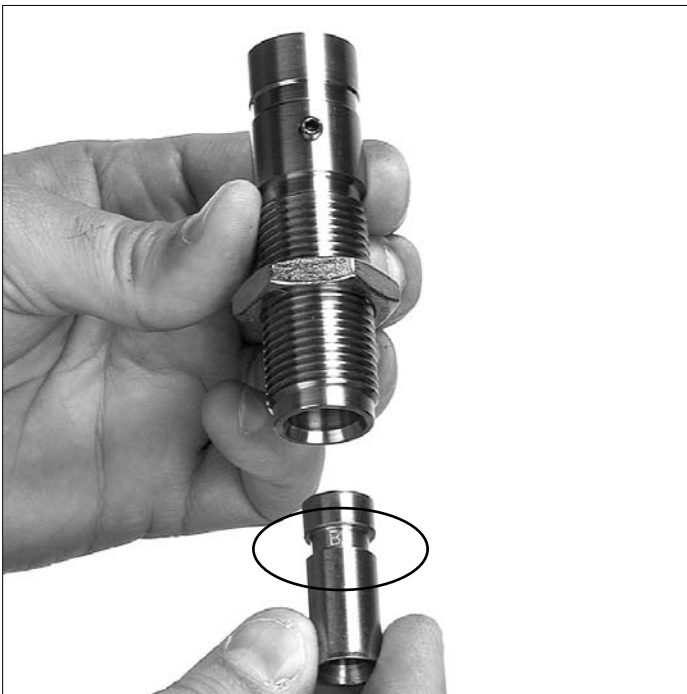
Figure 16 – The groove in the rifle powder funnel.
