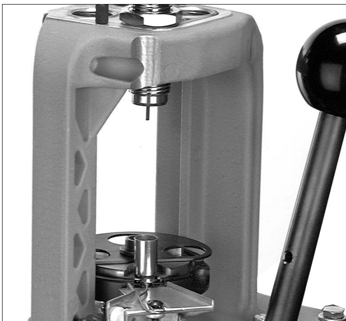
Figure 24 – Inserting an empty cartridge case in Station #1.
