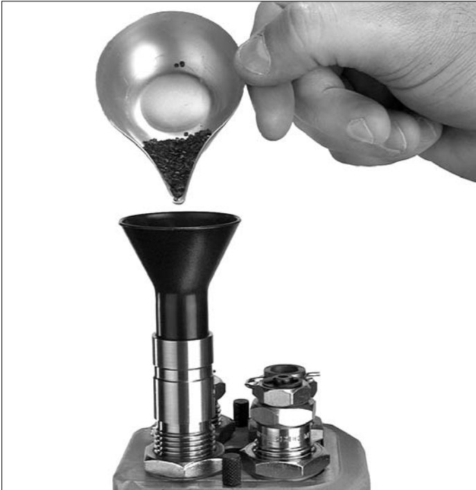
Figure 35 – Charging the case with powder at Station #2.
