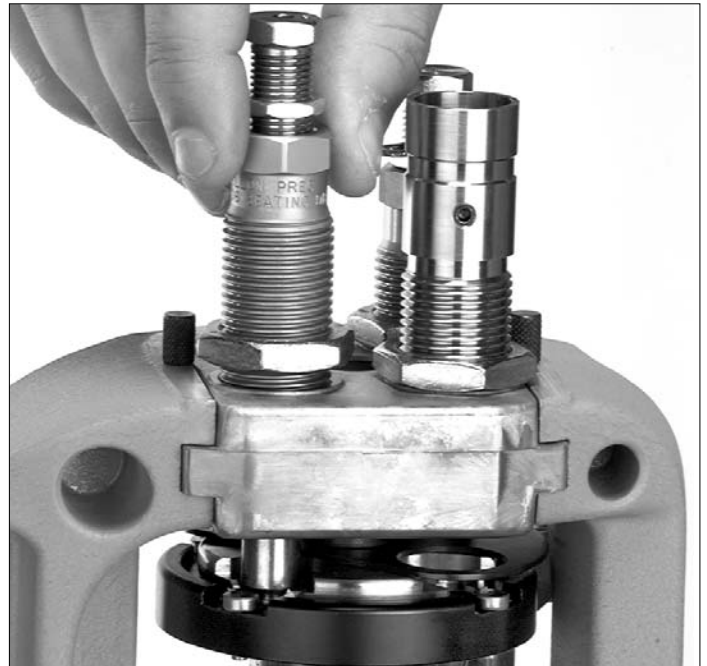
Figure 17 – Installing the bullet seating die in Station #3.
