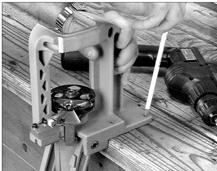
Figure 3 – Using the reloader as a template to mark your bench.
