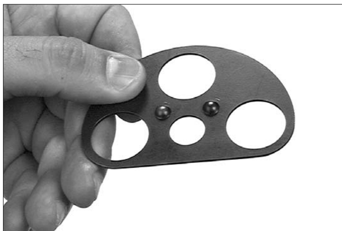
Figure 6 – Locator “dimples” on the AT 500 shellplate cover.
