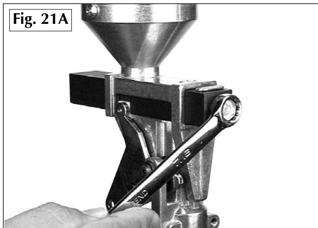
Station Two – Inside the powder die (#16744) you'll find the powder funnel Fig. 21 . This part uniforms the top of the shotshell hull and dispenses one charge of powder into the hull. The powder bar will need to be adjusted to the desired powder weight. Its important to use a quality powder scale to do this. Fig. 21A
