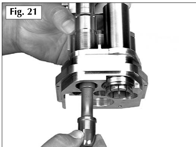
Station Two – Inside the powder die (#16744) you'll find the powder funnel Fig. 21 . This part uniforms the top of the shotshell hull and dispenses one charge of powder into the hull. The powder bar will need to be adjusted to the desired powder weight. Its important to use a quality powder scale to do this. Fig. 21A
