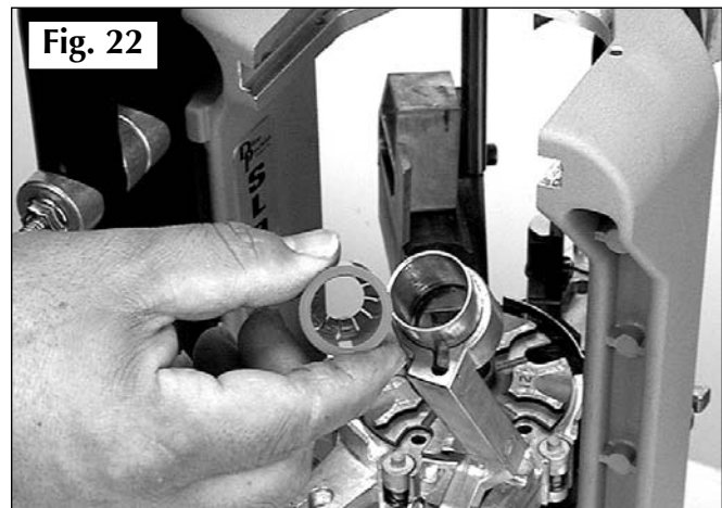
Station Three – Two operations occur here involving wad and shot insertion.
